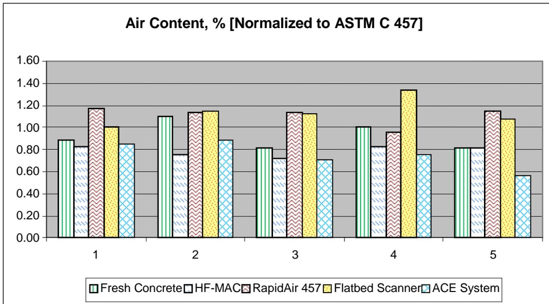
**Figure 10:** Results of air contents in five concrete cylinders measured in plastic concrete, by four different methods of automated image analysis, and by the modified point count method of ASTM C 457. The bottom diagram shows relative variations in air contents among four different image analyses methods after normalizing their results by the ASTM C 457 result.
