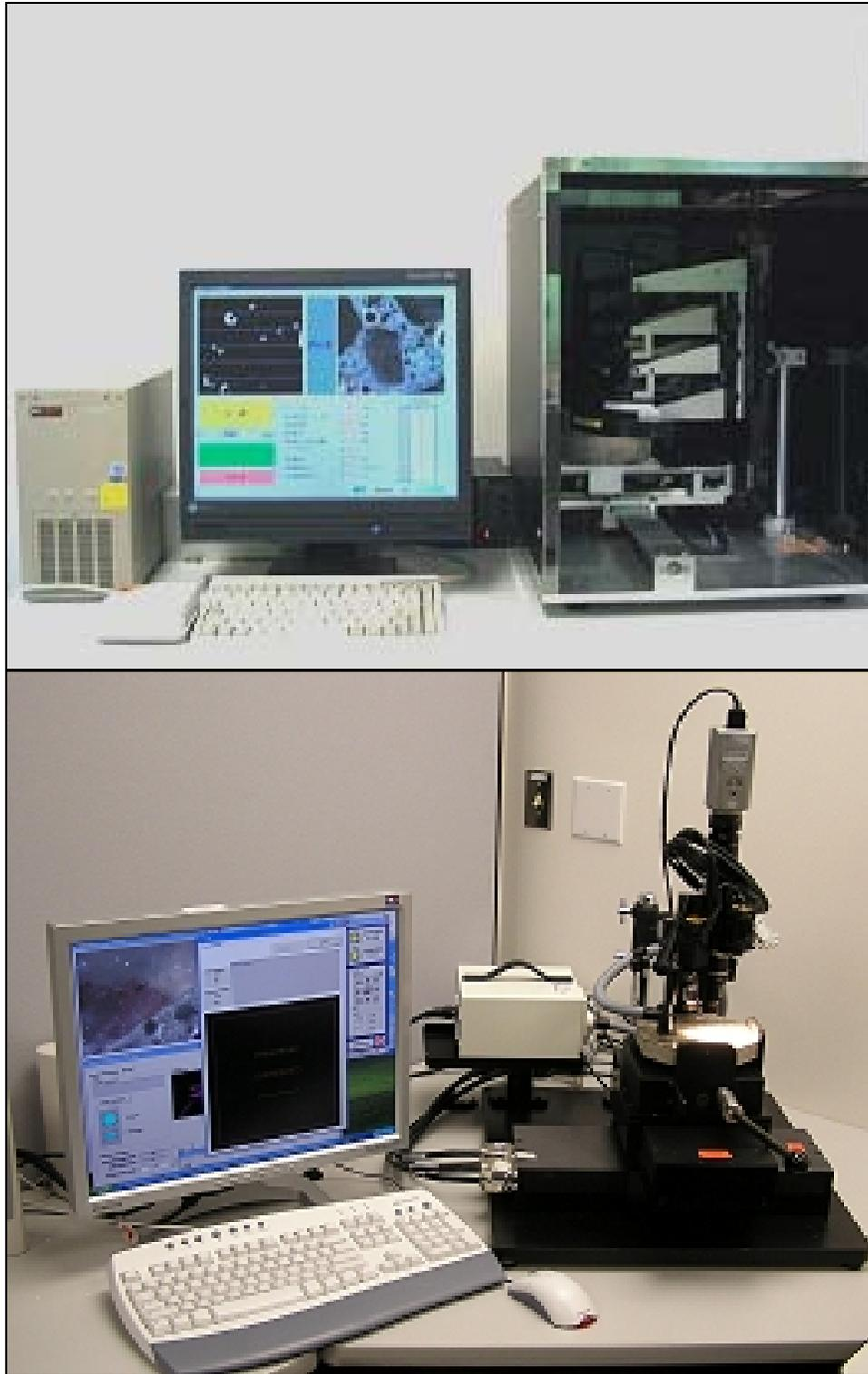
**Figure 7:** Instrument set up for HF-MAC01 method (top photo) and ACE system (bottom photo) neither of which require black-and-white contrast enhancement of the lapped section. Photos courtesy of Fast Corporation and NNSA-KCP.
