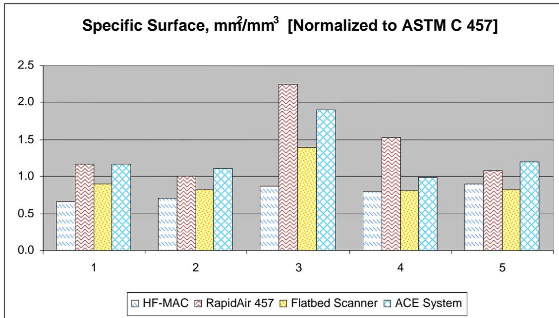
**Figure 12:** Results of specific surfaces of air void systems in five concrete cylinders measured by four different methods of automated image analysis, and by the modified point count method of ASTM C 457. The bottom diagram shows relative variations in a specific surface among four different image analysis methods after normalizing their results by the ASTM C 457 result.
