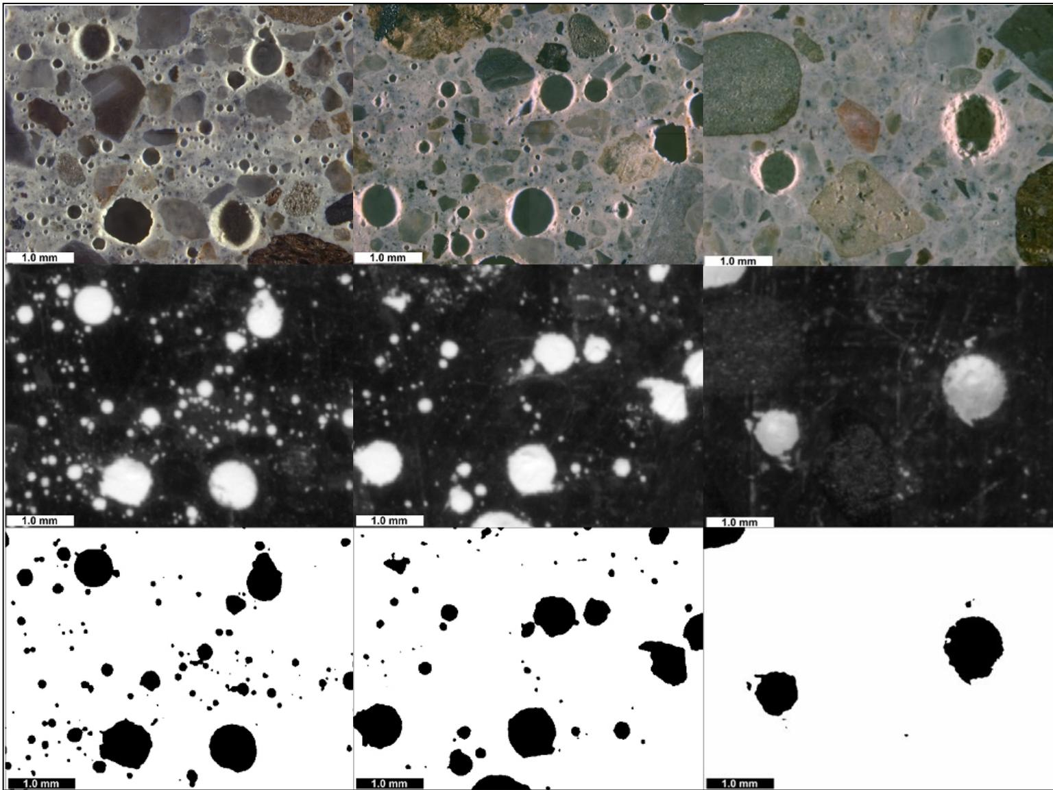
**Figure 9:** Samples 1(left photo), 2 (middle photo) and 3 (right photo) used for the flatbed scanner method; their determined air contents from the method are 9, 6, and 3.5 percent, respectively. In each photo, from top to bottom: A 2 x 2 mosaic of stereomicroscope image (as received), corresponding area from flatbed scanner image, and threshold image (Photos courtesy of Karl W. Peterson).
