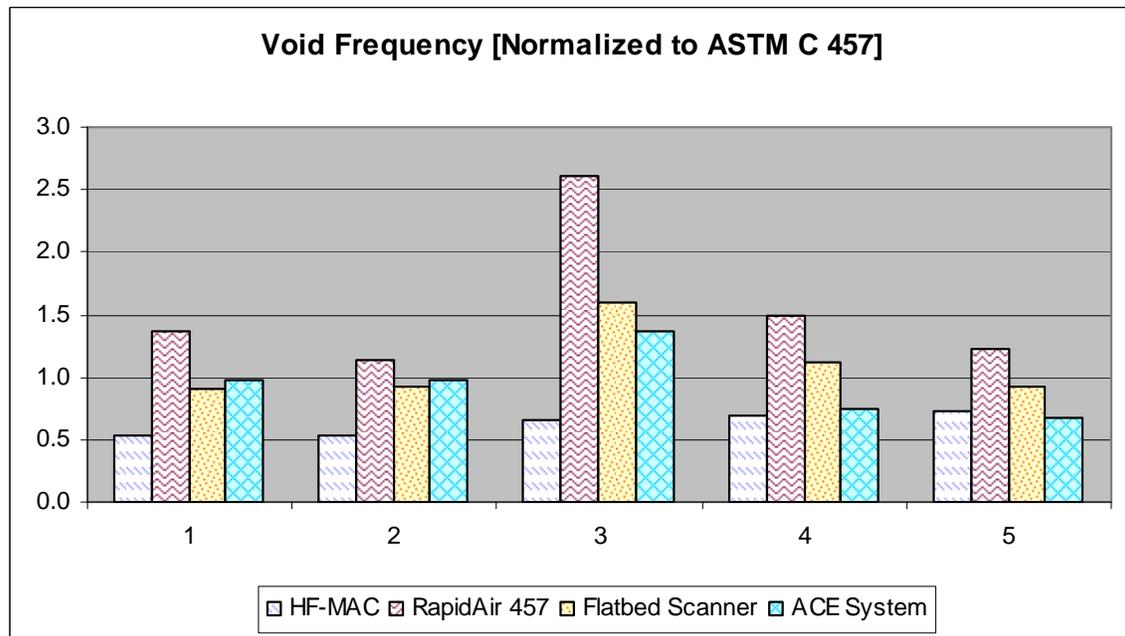
**Figure 11:** Results of void frequency of air void systems in five concrete cylinders measured by four different methods of automated image analysis, and by the modified point count method of ASTM C 457. The bottom diagram shows relative variations in void frequencies among four different image analysis methods after normalizing their results by the ASTM C 457 result.
