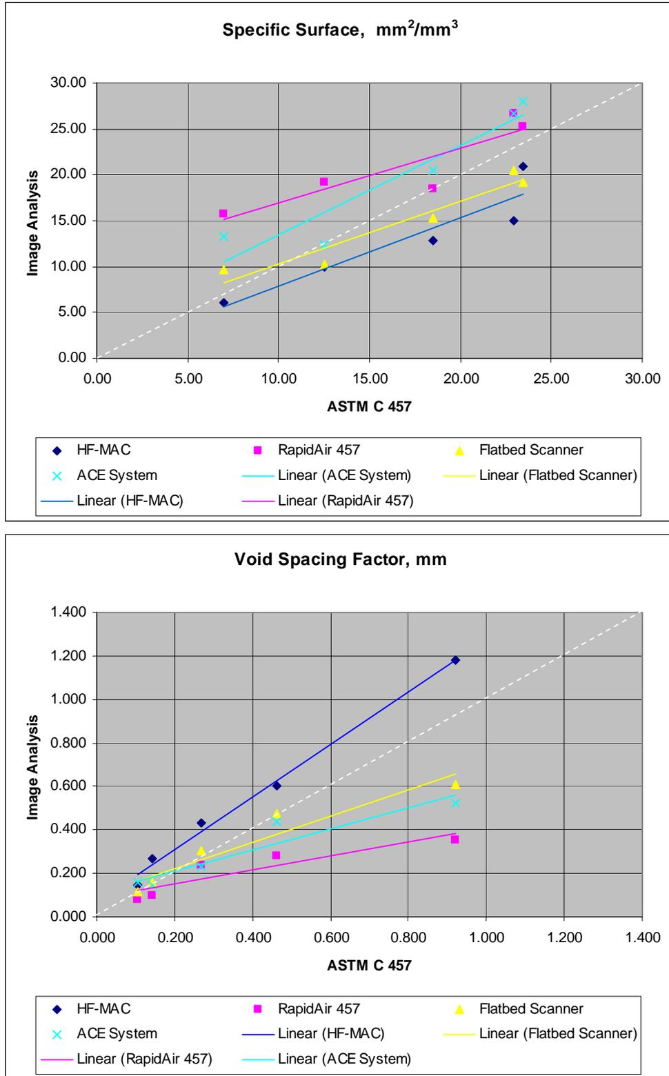
**Figure 15 (Cont'd):** Results of specific surface and void spacing factor of five samples determined from four different image analysis methods plotted against the corresponding average values determined from the manual modified point methods of ASTM C 457 by two laboratories.
