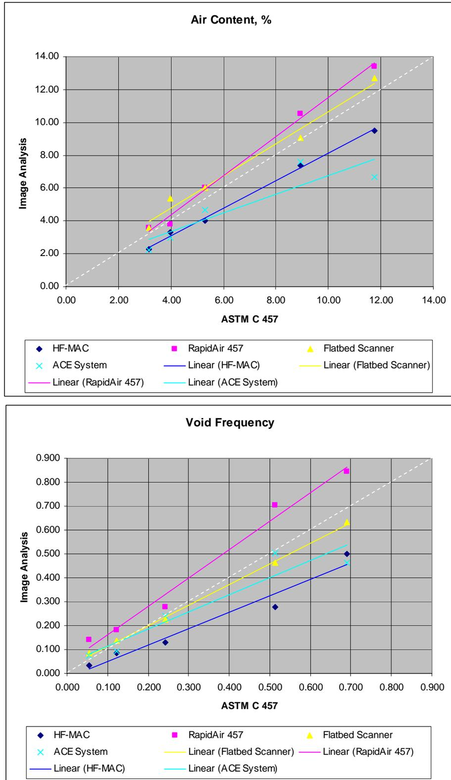
**Figure 15:** Results of air contents and void frequency of five samples determined from four different image analysis methods plotted against the corresponding average values determined from the manual modified point methods of ASTM C 457 by two laboratories.
