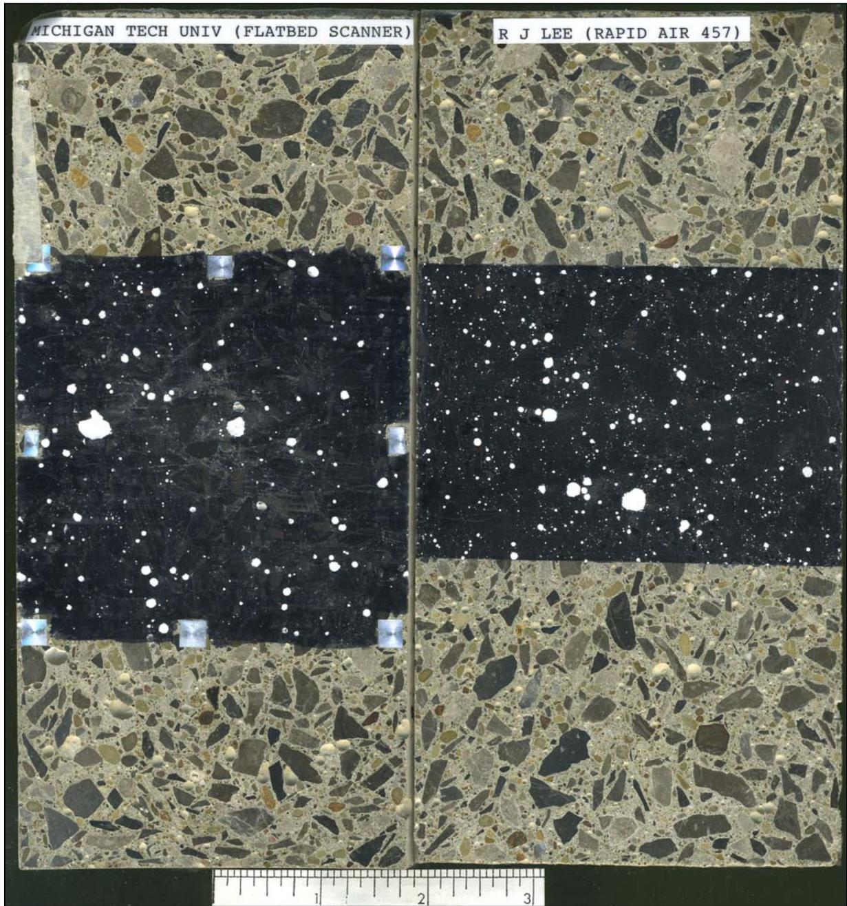
**Figure 8:** Black and white contrast enhancements on the lapped sections for the flatbed scanner method (left photo, Cylinder 3) and RapidAir 457 method (right photo, Cylinder 4).
