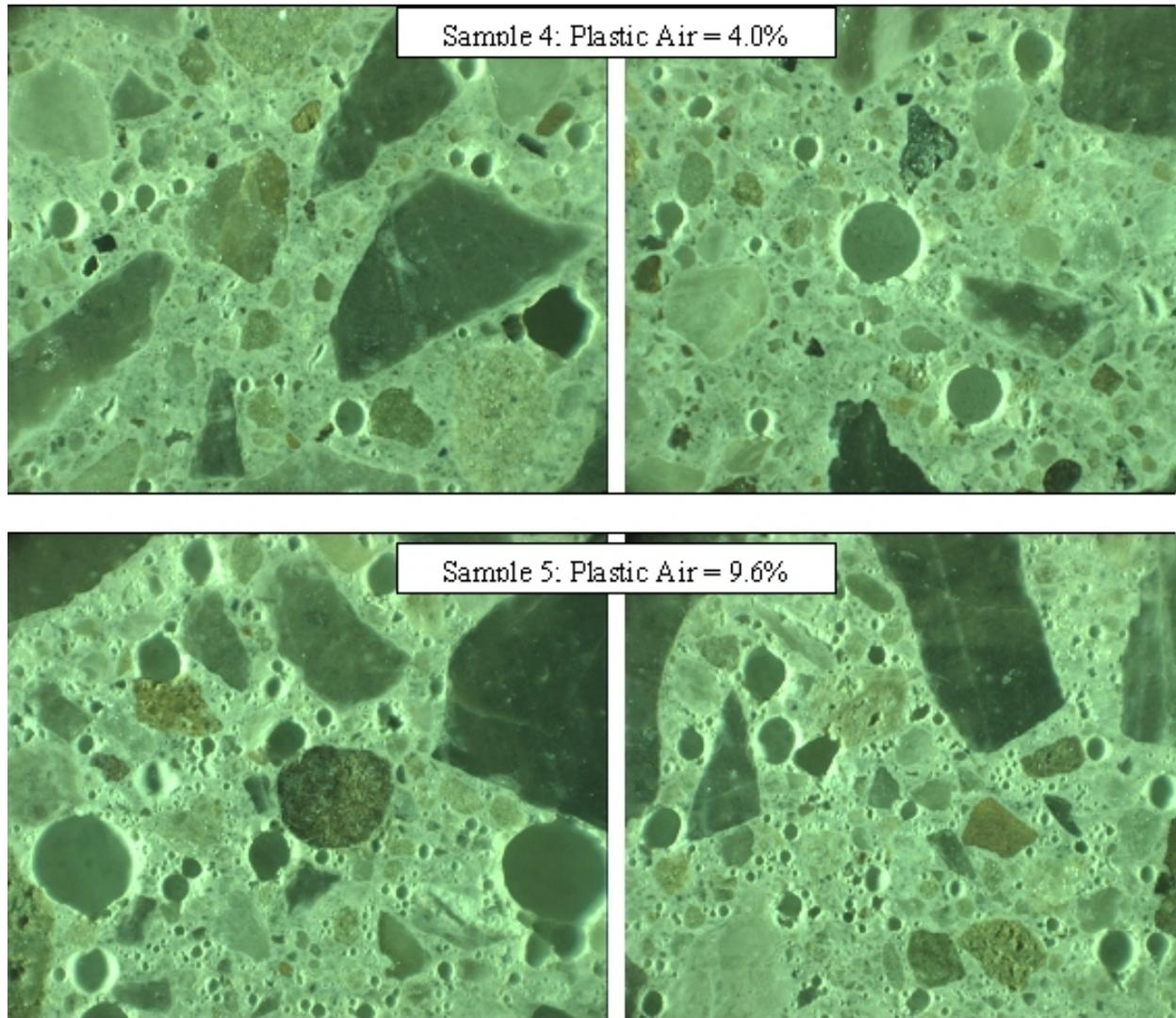
**Figure 3:** Photomicrographs of lapped sections of five concrete cylinders after sectioning and lapping at the CMC Laboratory. “Plastic air” represents air contents measured in the fresh concrete mixtures after mixing, and prior to preparing the cylinders. Field width of each photo is 10 mm.
