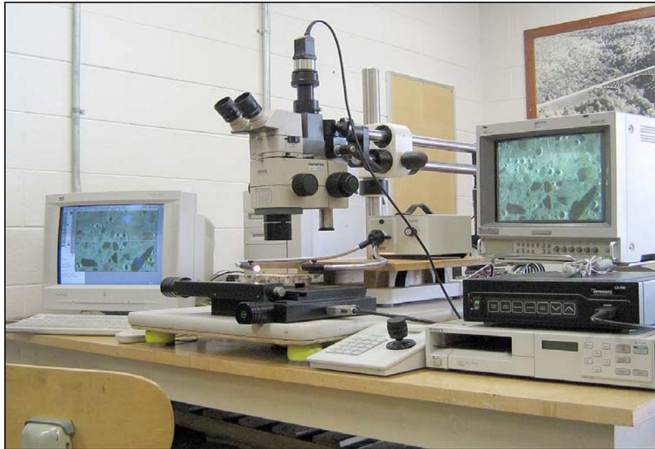
**Figure 5:** Instrument setup for the modified point count (manual) method of ASTM C 457 used in Michigan Technological University.
