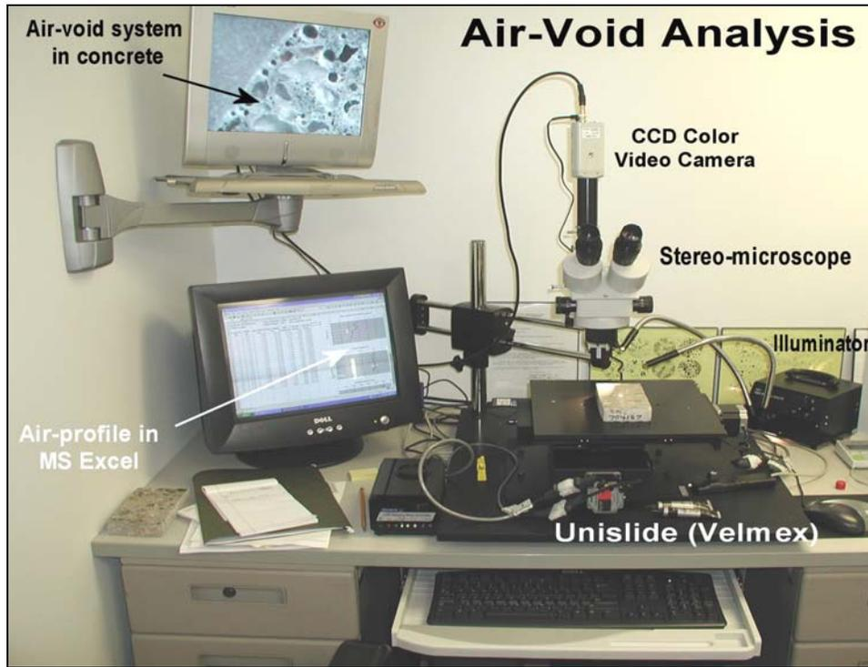
**Figure 4:** Instrument setup for the modified point count (manual) method of ASTM C 457 used in the laboratory of Construction Materials Consultants, Inc.
