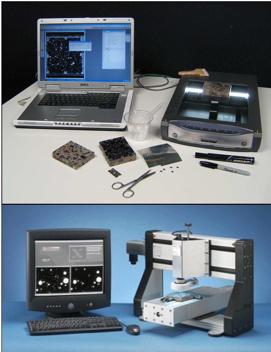
**Figure 6:** Instrument setup for the flatbed scanner method (top photo) and the RapidAir 457 method (bottom photo) both of which require a black and white contrast enhancement of the lapped section being scanned. Photos courtesy of Michigan Technological University and Concrete Experts International.
