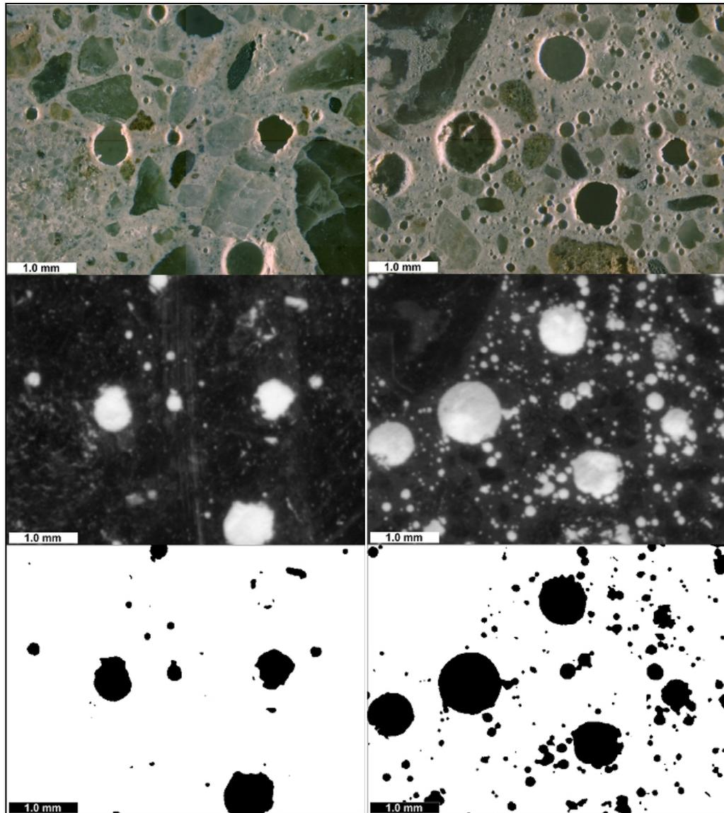
**Figure 9 (Cont'd):** Samples 4 (left photo) and 5 (right photo) used for flatbed scanner method; their determined air contents from the method are 5.3 and 12.7 percent. In each photo, from top to bottom: A 2 x 2 mosaic of stereomicroscope image (as received), corresponding area from flatbed scanner image, and threshold image (Photo courtesy of Karl W. Peterson).
