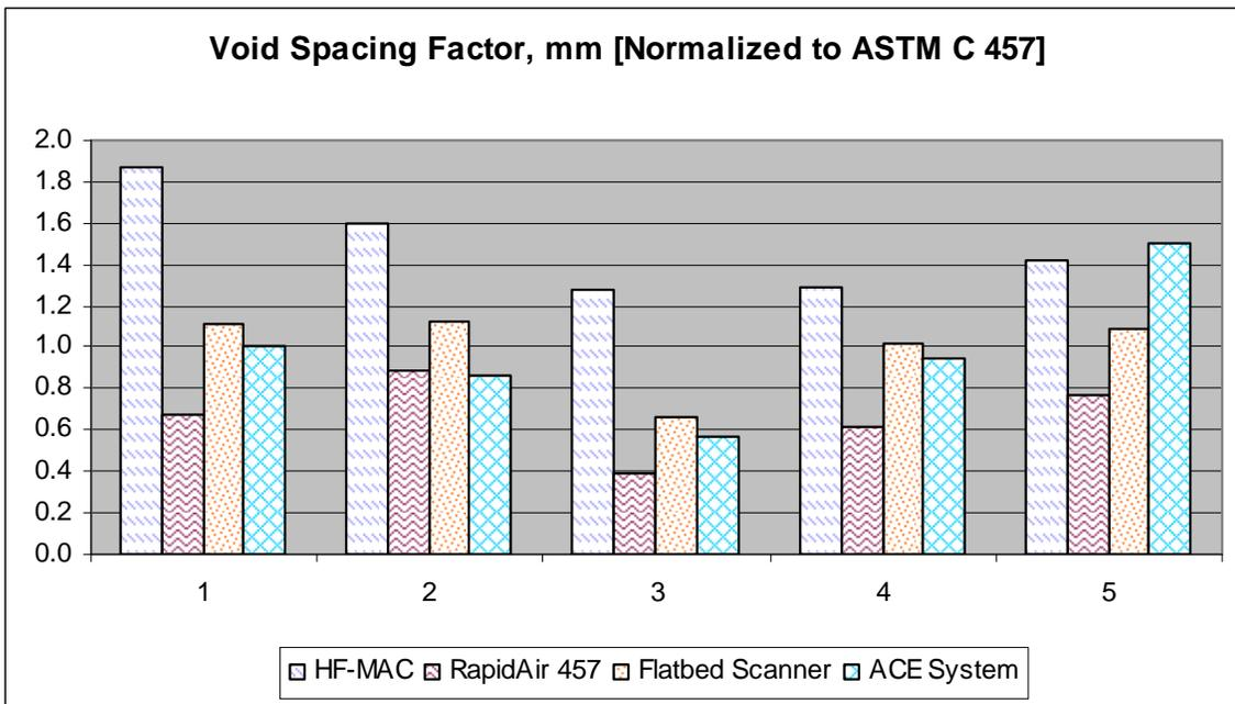
**Figure 13:** Results of void spacing factors of air void systems in five concrete cylinders measured by four different methods of automated image analysis, and by the modified point count method of ASTM C 457. The bottom diagram shows relative variations in void spacing factor among four different image analysis methods after normalizing their results by the ASTM C 457 result.
