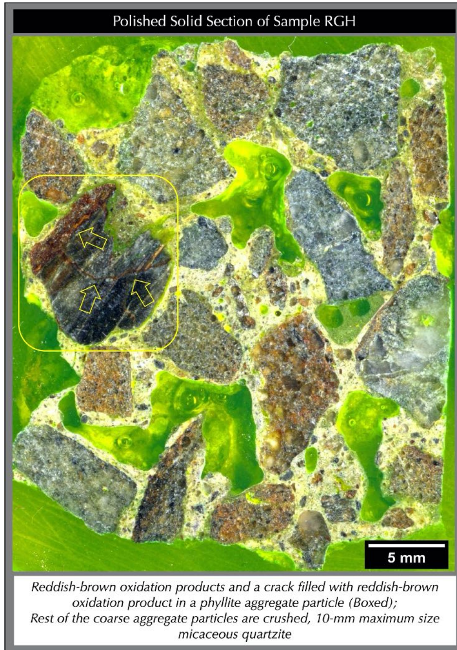
Figure 10: Polished section of sample RGH showing only one potentially deleterious phyllite coarse aggregate with reddish-brown oxidation products of iron and associated microcracks, which are also filled with the oxidation products (marked by arrows). Rest of the coarse aggregate particles are crushed micaceous quartzite , which are dense, hard, equigranular to elongated, massive quartzitic (granoblastic) textured mass of equigranular grains of major amount of quartz, subordinate feldspar (albite), and parallel bands of muscovite and chlorite, having a nominal maximum size of 10 mm. Interstitial paste in the mortar fraction shows beige color tone. Coarse irregular-shaped interstitial voids are calculated (from ImageJ) to be less than 10 percent.
