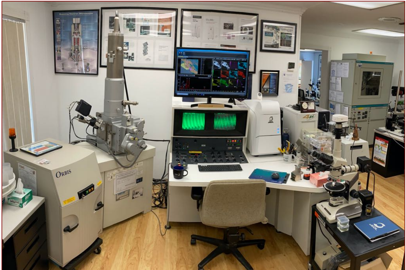
Figure 7: JEOL Neoscope JCM-7000 benchtop and CamScan Series 2 floor model scanning electron microscopes in CMC used to examine samples at noticeably higher magnifications than optical microscopes along with detailed microstructural and microchemical analyses.
