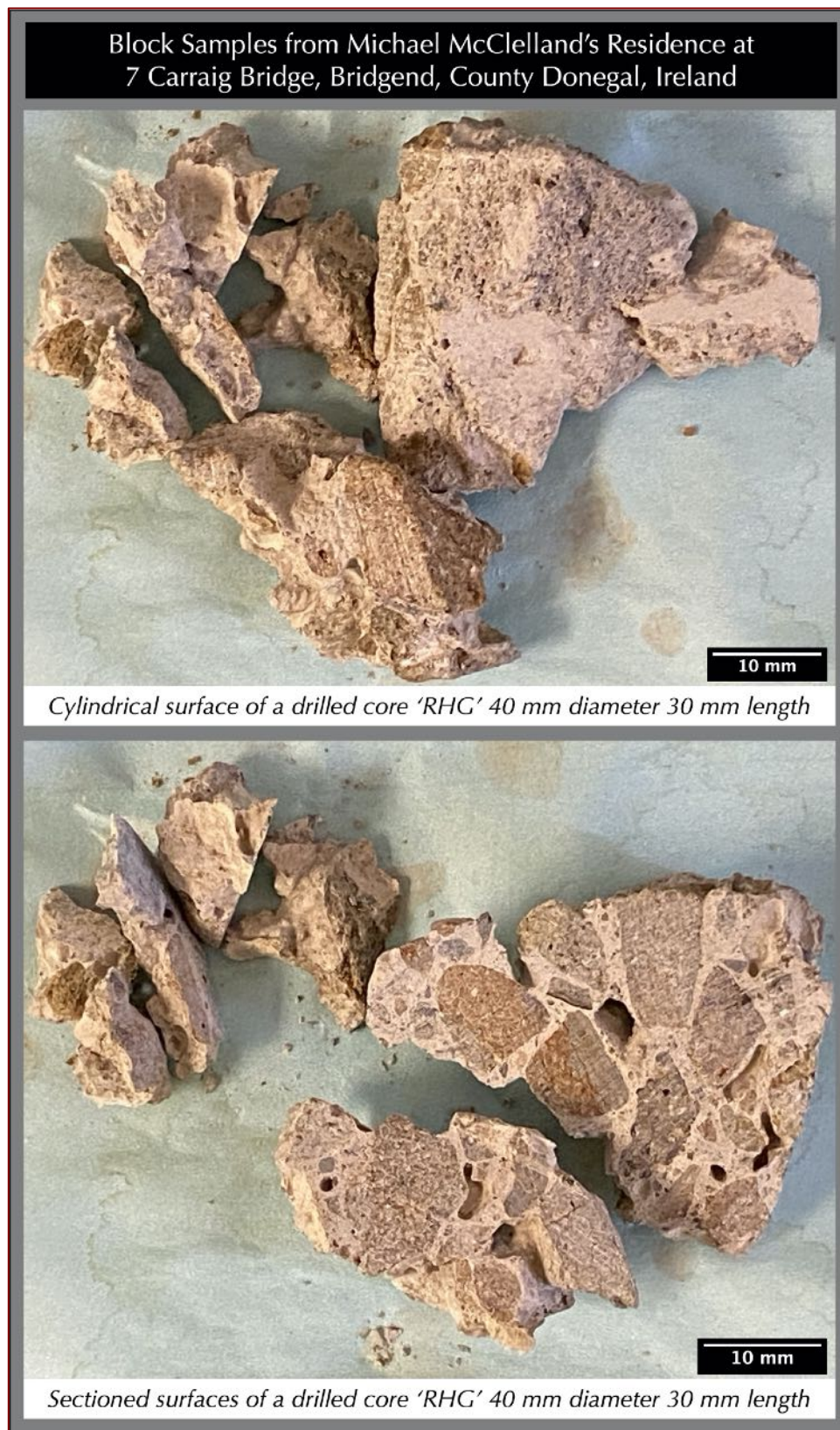
Figure 5: Cylindrical (top) and cross sectioned (bottom) surfaces of drilled core 'RHG' showing crushed micaceous quartzite aggregate, interstitial paste, and coarse voids.
