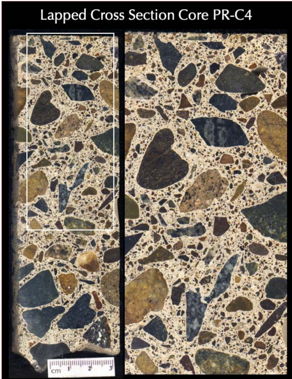
Figure 13: Lapped cross section of Core PR-C4 showing: (a) a thin paint coat at the top well-bonded to the underlying concrete having a nominal thickness of < 1 mm; (b) the main concrete body containing crushed volcanic and volcanoclastic gravel coarse aggregate where aggregate particles are subrounded to subangular, dense, variably colored, well-graded, and well-distributed, natural siliceous sand and finer fractions of volcanic rocks and minerals in fine aggregate, all dispersed in a Portland cement paste; and, (c) the overall sound (visually crack-free), dense, well-consolidated nature of the concrete in the body. The boxed area at left is enlarged at right.
