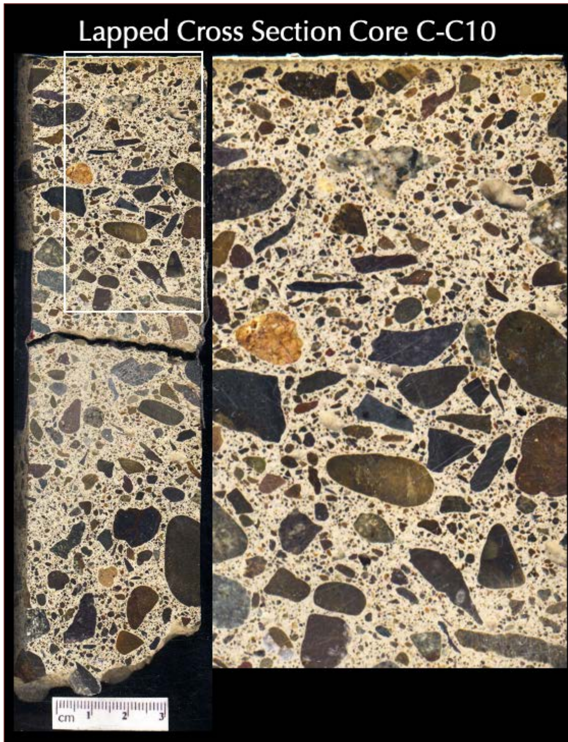
Figure 10: A second lapped cross section of Core C-C10 showing: (a) a thin paint coat at the top well-bonded to the underlying concrete having a nominal thickness of < 1 mm; (b) the main concrete body containing crushed volcanic and volcaniclastic gravel coarse aggregate where aggregate particles are subrounded to subangular, dense, variably colored, well-graded, and well-distributed, natural siliceous sand and finer fractions of volcanic rocks and minerals in fine aggregate, all dispersed in a Portland cement paste; and, (c) the overall sound (visually crack-free), dense, well-consolidated nature of the concrete in the body. The boxed area at left is enlarged at right. The beige discoloration of paste at the top 10 mm beneath the protective coating is due to atmospheric carbonation of paste prior to the application of protective coating.
