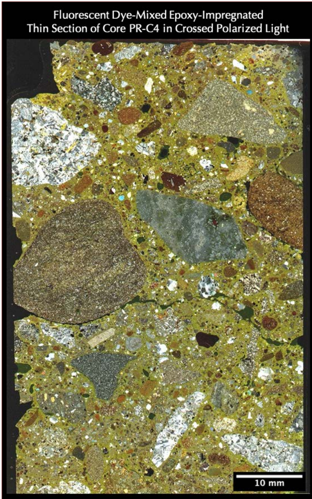
Figure 34: Fluorescent dye-mixed epoxy-impregnated thin section of Core PR-C4 seen in the crossed polarized light (XPL) mode by scanning the section in a film scanner sandwiched between two polarizing filters at perpendicular positions showing:
