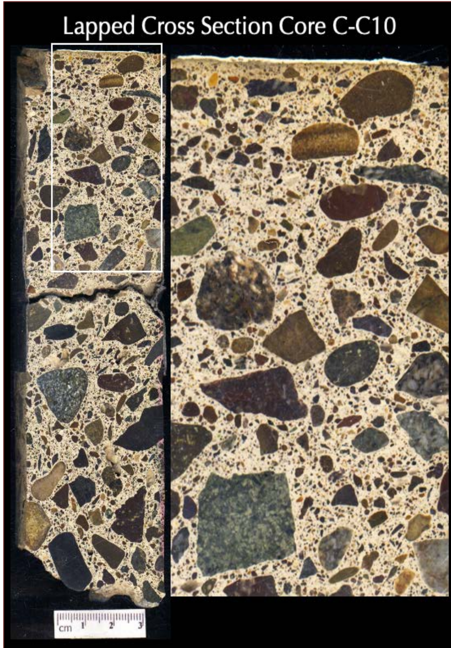
Figure 9: Lapped cross section of Core C-C10 showing:
