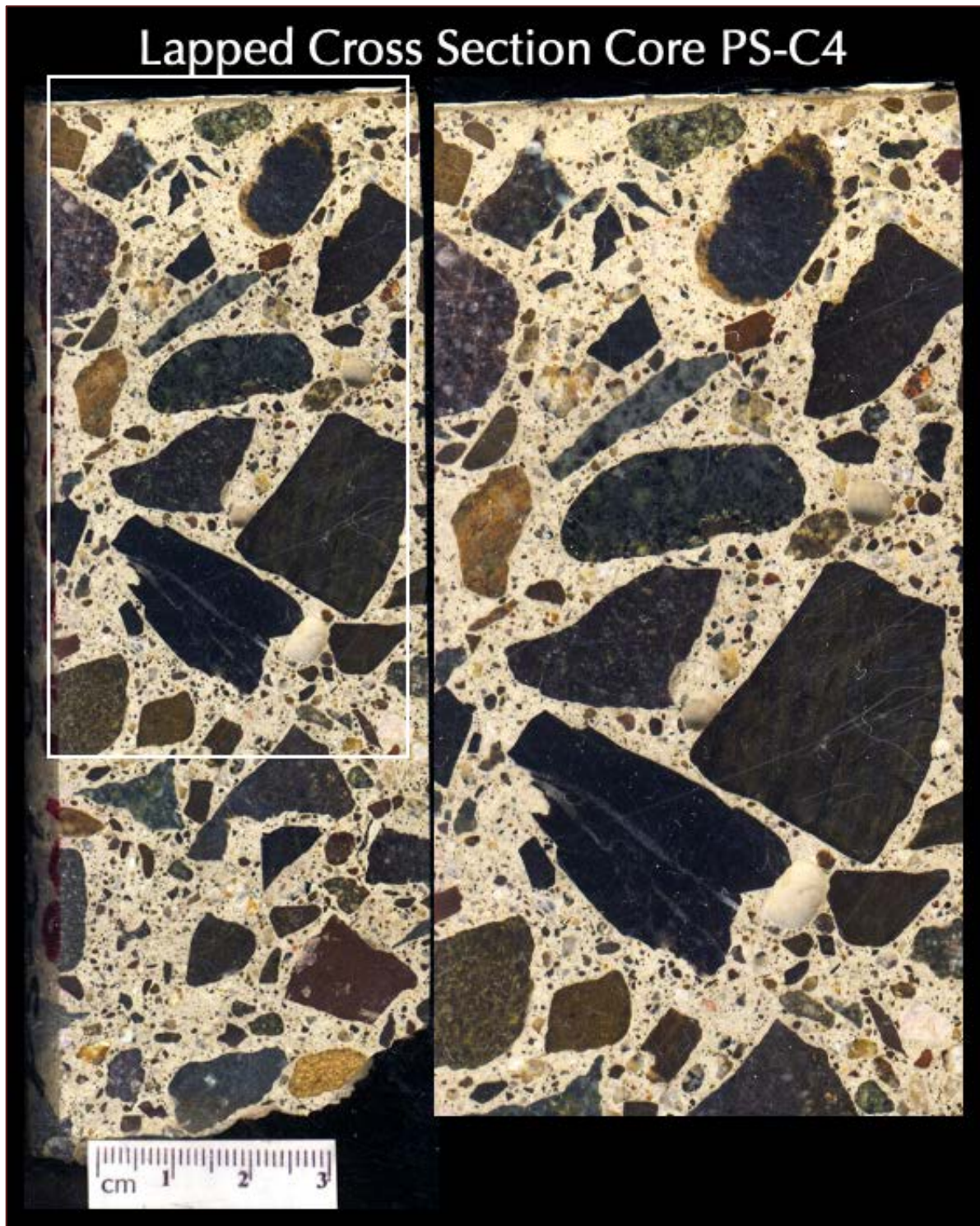
Figure 16: A second lapped cross section of Core PS-C4 showing: (a) a thin paint coat at the top well-bonded to the underlying concrete having a nominal thickness of < 1 mm; (b) the main concrete body containing crushed volcanic and volcaniclastic gravel coarse aggregate where aggregate particles are subrounded to subangular, dense, variably colored, well-graded, and well-distributed, natural siliceous sand and finer fractions of volcanic rocks and minerals in fine aggregate, all dispersed in a Portland cement paste; and, (c) the overall sound (visually crack-free), dense, well-consolidated nature of the concrete in the body. The boxed area at left is enlarged at right.
