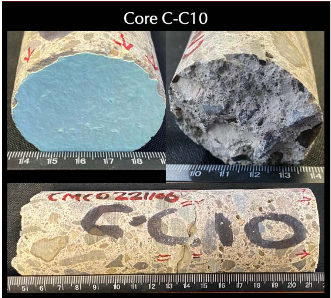
Figure 4: Shown are the exterior painted surface (top left), interior fractured end (top right) and side cylindrical surfaces of the Core C-C10 from Channel.
