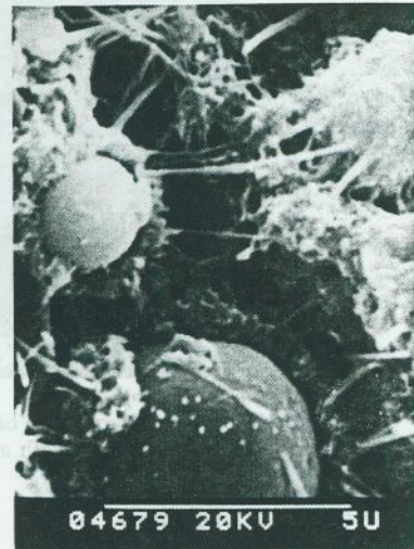
FIG. 18. Particles of fly ash in a Portland cement paste with needle-like crystals of calcium silicate hydrates linking the spheres to the hydrated gel.
