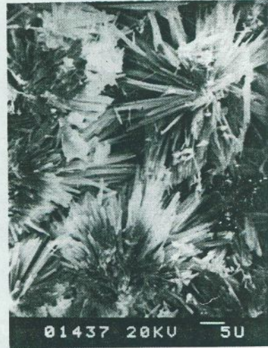
FIG. 14. A cluster of radiating growths of ettringite needles within hydrated paste.
