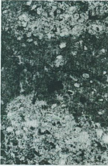
FIG. 21. This photograph shows a fine crack across the centre. The paste on either side of the crack has been recrystallized as a result of the passage of moisture along the crack. Width of photograph = 0.5 mm.
