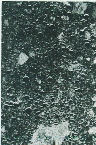
FIG. 28. A typical view of Portland cement paste exhibiting air entrainment. Width of photograph = 20 mm.
