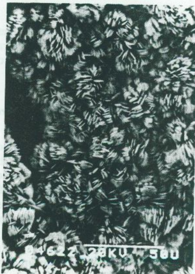
FIG. 17. Alkali-silicate gel which has become crystallized as a result of dehydration.
