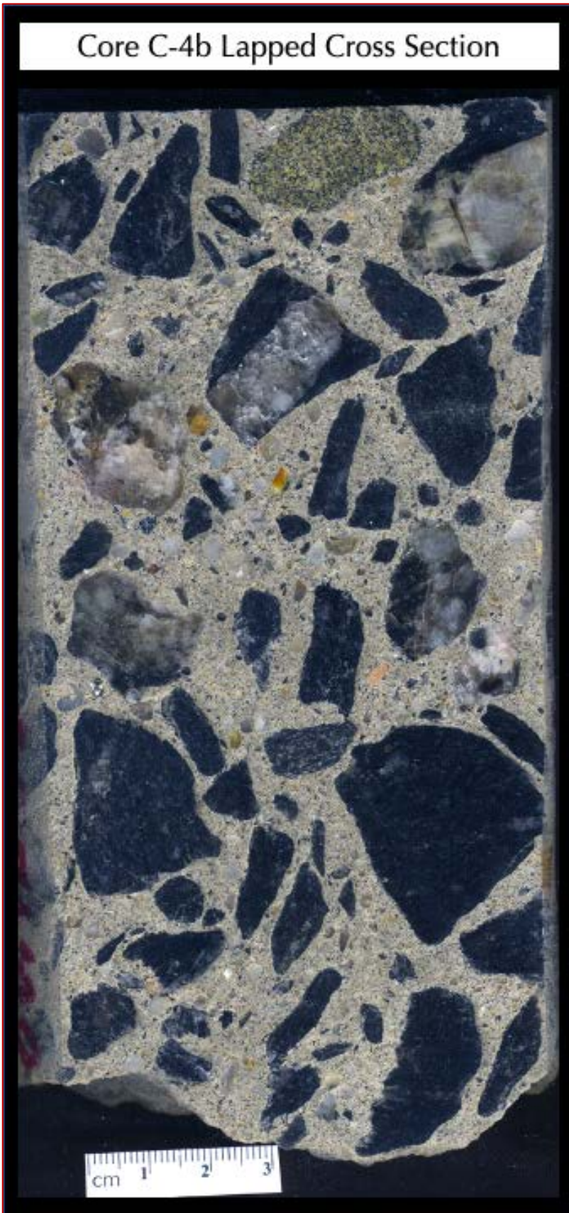
Figure 23: Lapped cross section of middle portion of Core C-4b having a saw-cut end at one side and a fresh fractured end at the opposite side, showing:
