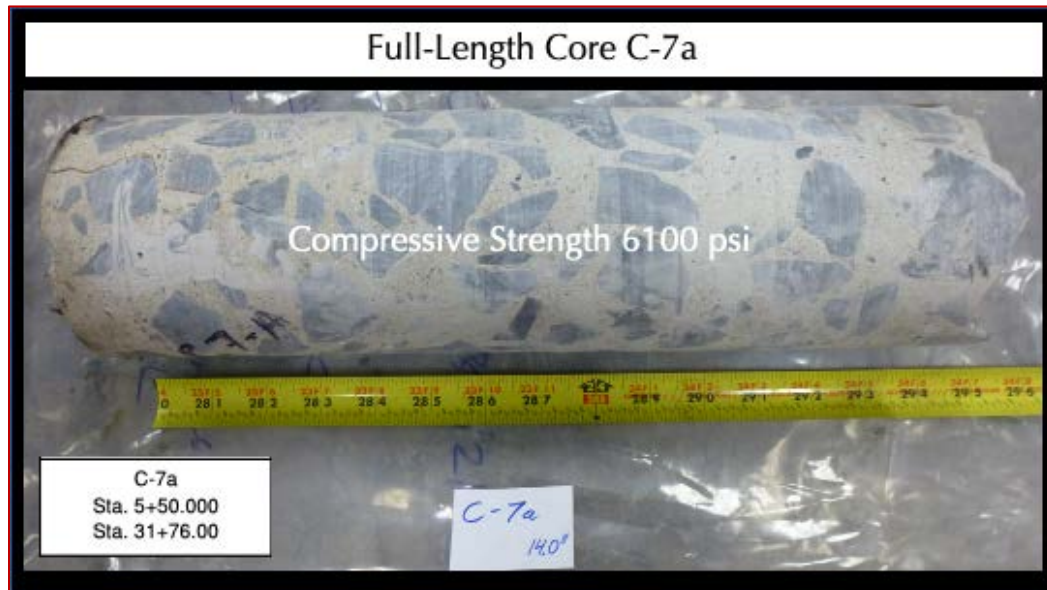
Figure 16: Full lengths of Core C-7a, and compressive strength result.
