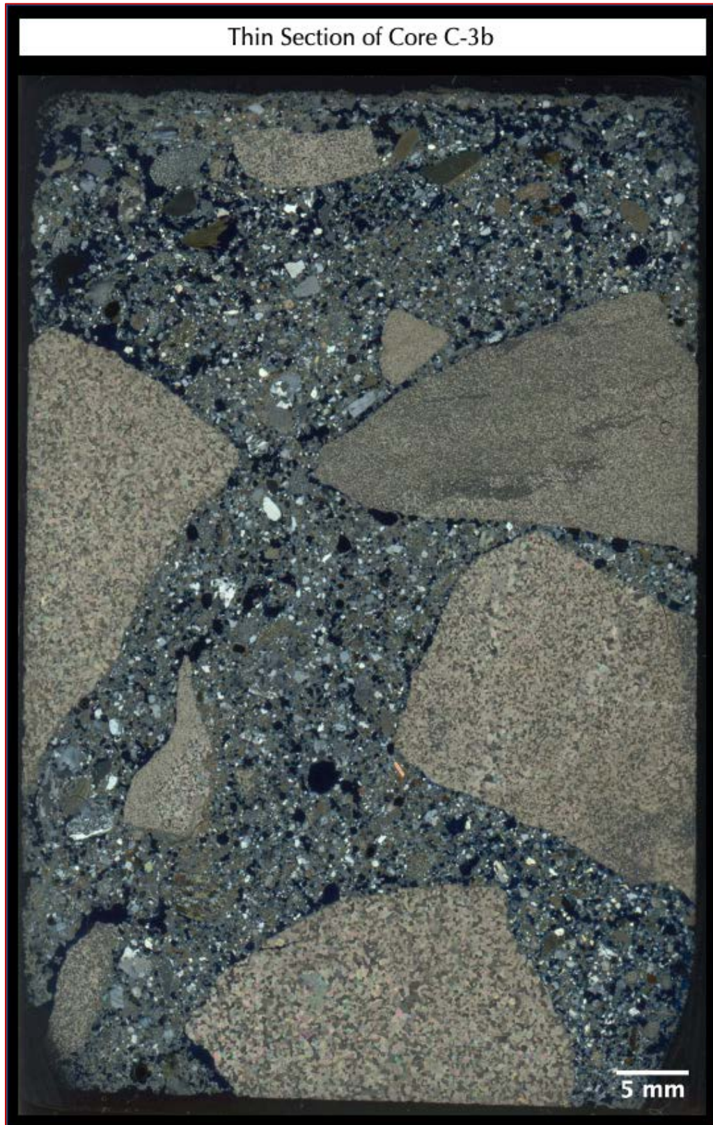
Figure 32: Enlarged view of a 50 mm × 75 mm size blue dye-mixed epoxy-impregnated thin section of Core C-3b, shown in cross polarized light mode by scanning the thin section on a flatbed scanner with two perpendicular polarizing filters between the thin section. The image highlights crushed limestone-dolomite coarse aggregate and an interstitial mortar fraction of natural siliceous-argillaceous sand fine aggregate and Portland cement paste.
