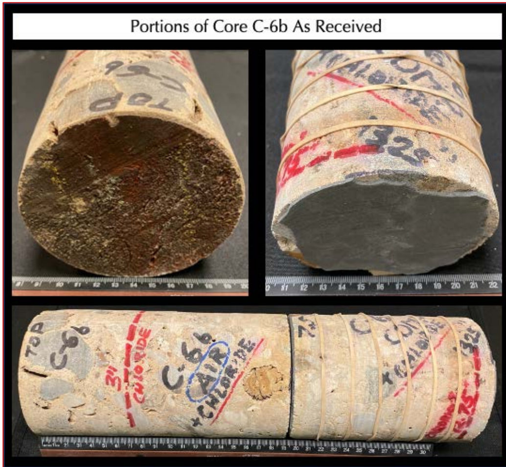
Figure 15: Portions of core as received from C-6b and the requested testing.
