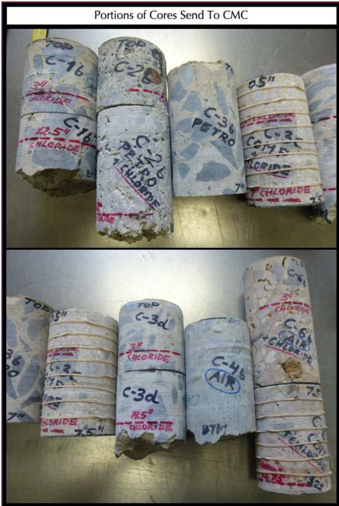
Figure 17: Portions of cores received for petrographic examinations (Cores C-2b and 3b), air-void analysis (Cores C-4b and 6b), and depth markings for water-soluble chloride contents at two depths (Cores C-1b, 2b, 3c, 3d, and 6b).
