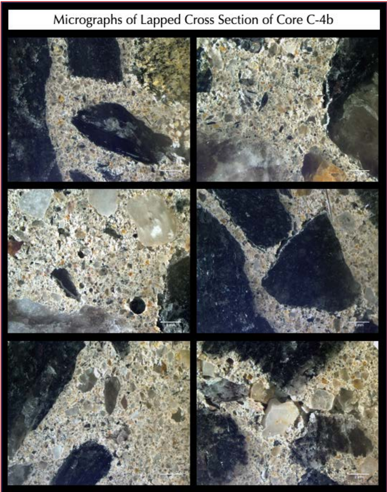
Figure 27: Micrographs of lapped cross section of Core C-4b showing: (a) the overall non-air-entrained nature of concrete having a few discrete, spherical and near-spherical entrapped air bubbles, and (b) overall porous but well-consolidated nature of concrete.
