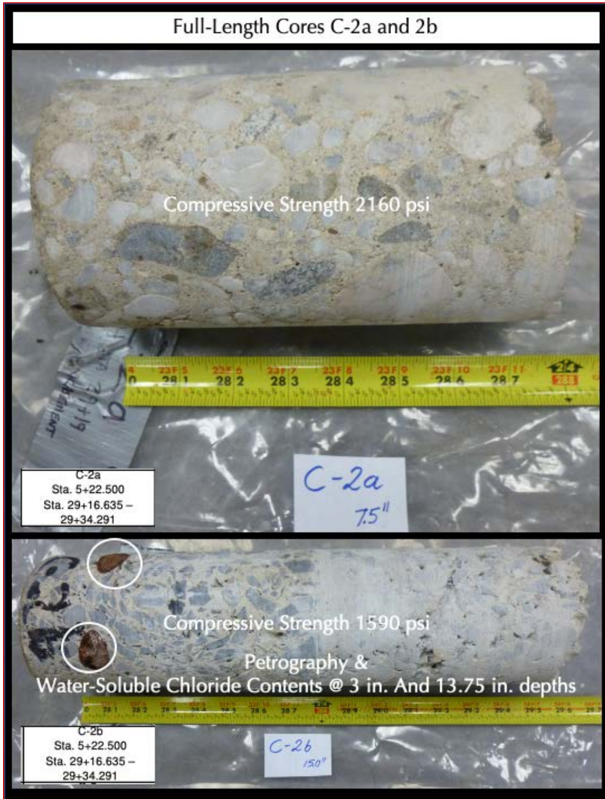
Figure 3: Full lengths of Cores C-2a and 2b, type of testing done, and compressive strength results.
