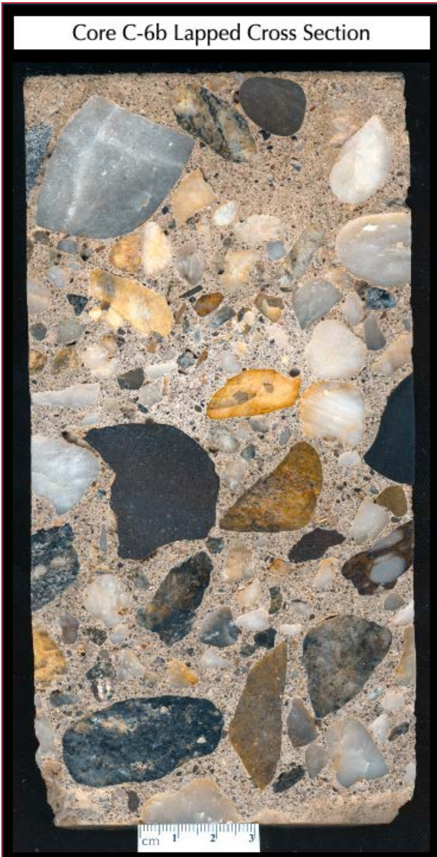
Figure 24: Lapped cross section of top portion of Core C-6b having a weathered exposed end at one side and a saw-cut end at the opposite side, showing:
