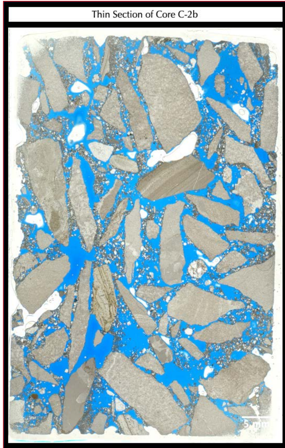
Figure 29: Enlarged view of a 50 mm × 75 mm size blue dye-mixed epoxy-impregnated thin section of Core C-2b, shown in plane polarized light mode by scanning the thin section on a flatbed scanner with a polarizing filter. The image highlights abundant coarse entrapped air voids in the concrete due to inadequate filling of interstitial spaces between elongated crushed limestone-dolomite coarse aggregate leaving only minor mortar fraction of natural siliceous-argillaceous sand fine aggregate and Portland cement paste.
