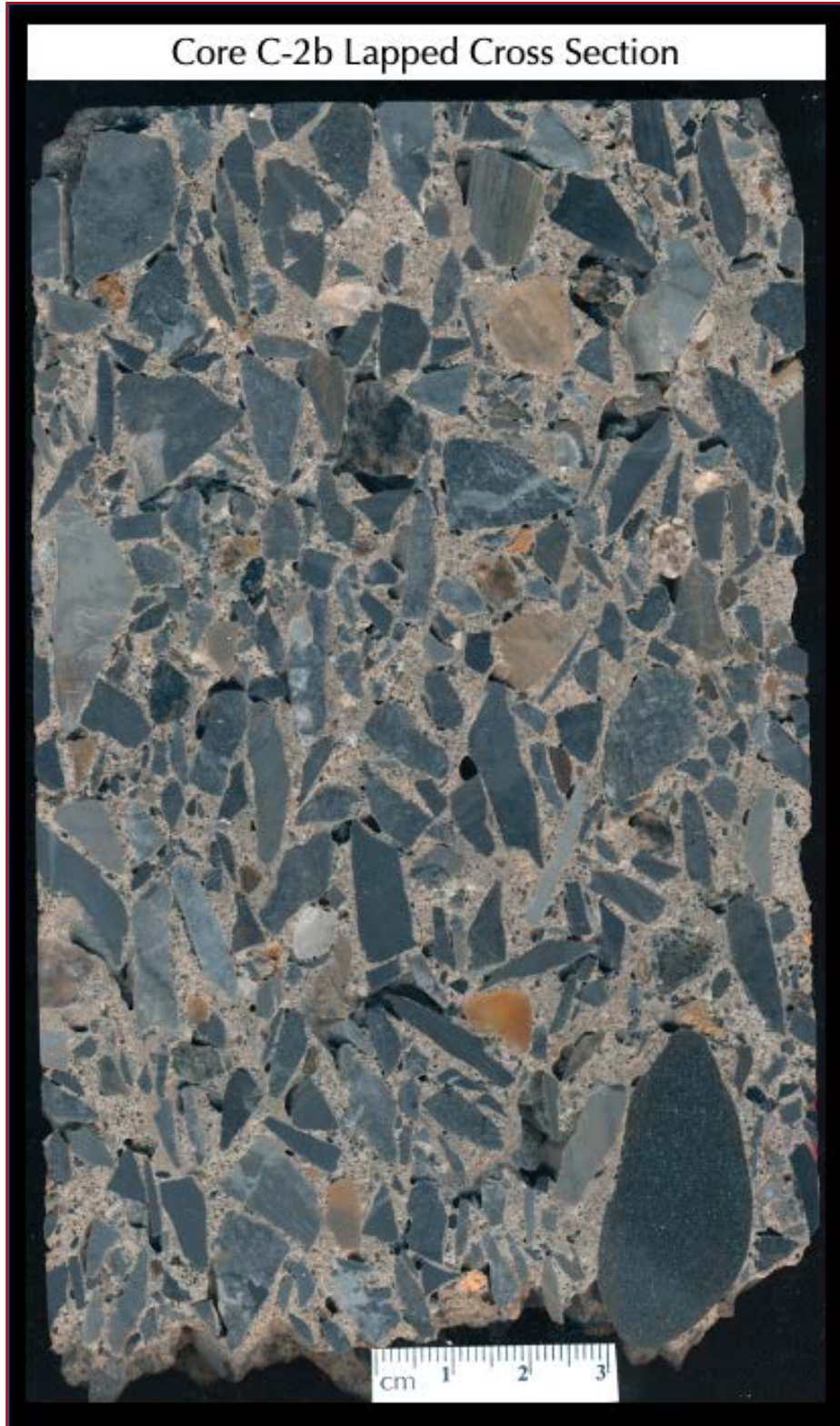
Figure 21: Lapped cross section of a middle portion of Core C-2b having a saw-cut end at one side and fractured end at the opposite side, showing:
