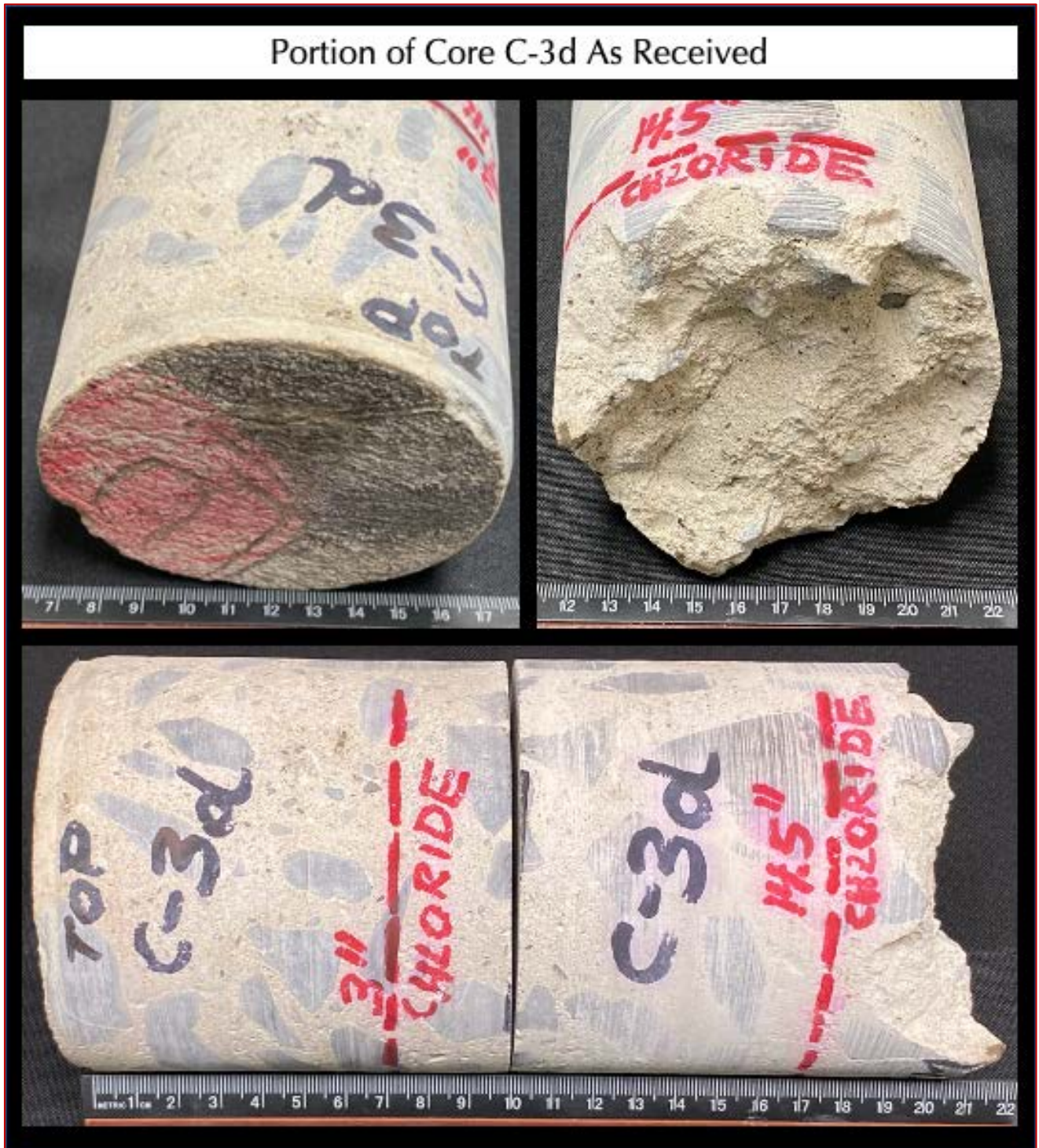
Figure 10: Portions of core as received from C-3d and the requested testing.
