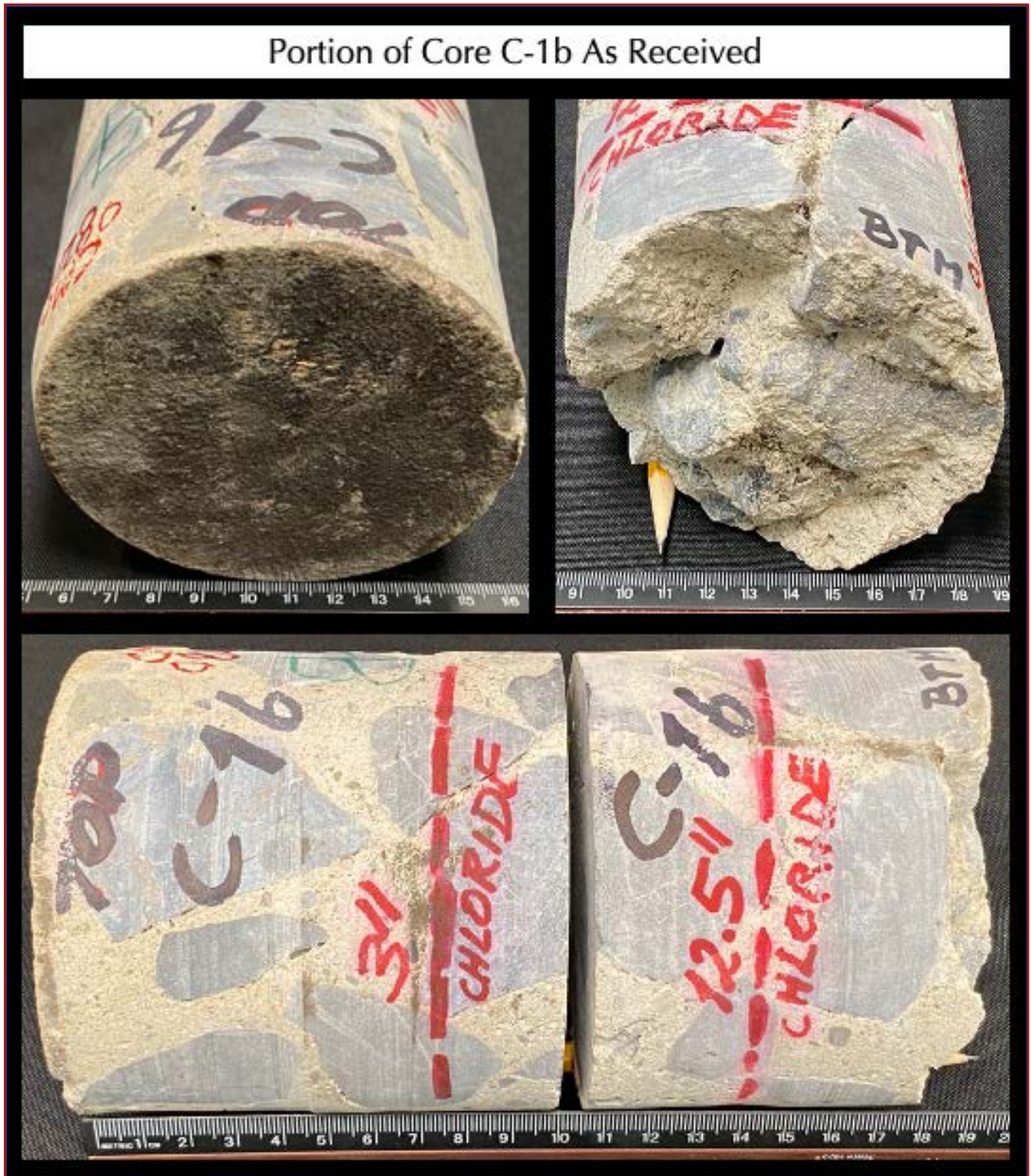
Figure 2: Portions of core as received from C-1b and the requested testing.
