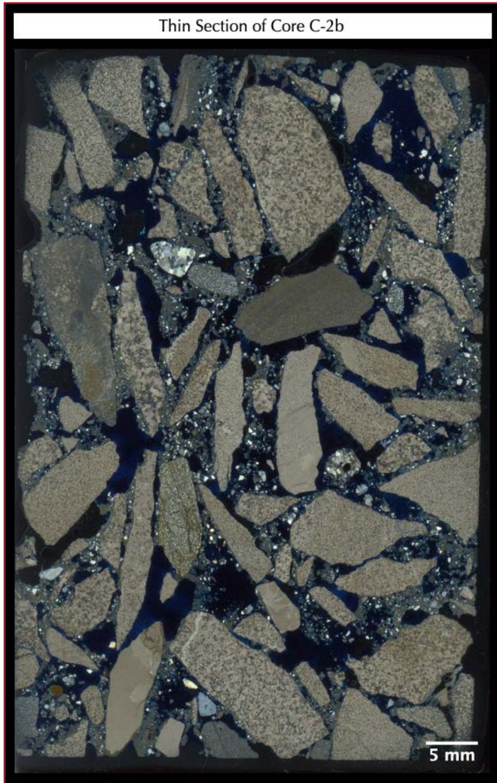
Figure 30: Enlarged view of a 50 mm × 75 mm size blue dye-mixed epoxy-impregnated thin section of Core C-2b, shown in crossed polarized light mode by scanning the thin section on a flatbed scanner with two perpendicular polarizing filters between the thin section. The image highlights crushed limestone-dolomite coarse aggregate leaving only minor mortar fraction of natural siliceous-argillaceous sand fine aggregate and Portland cement paste.
