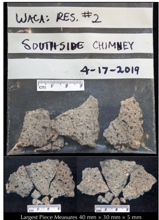
Figure 2: Mortar sample from southside of chimney, as received in multiple fragments.
