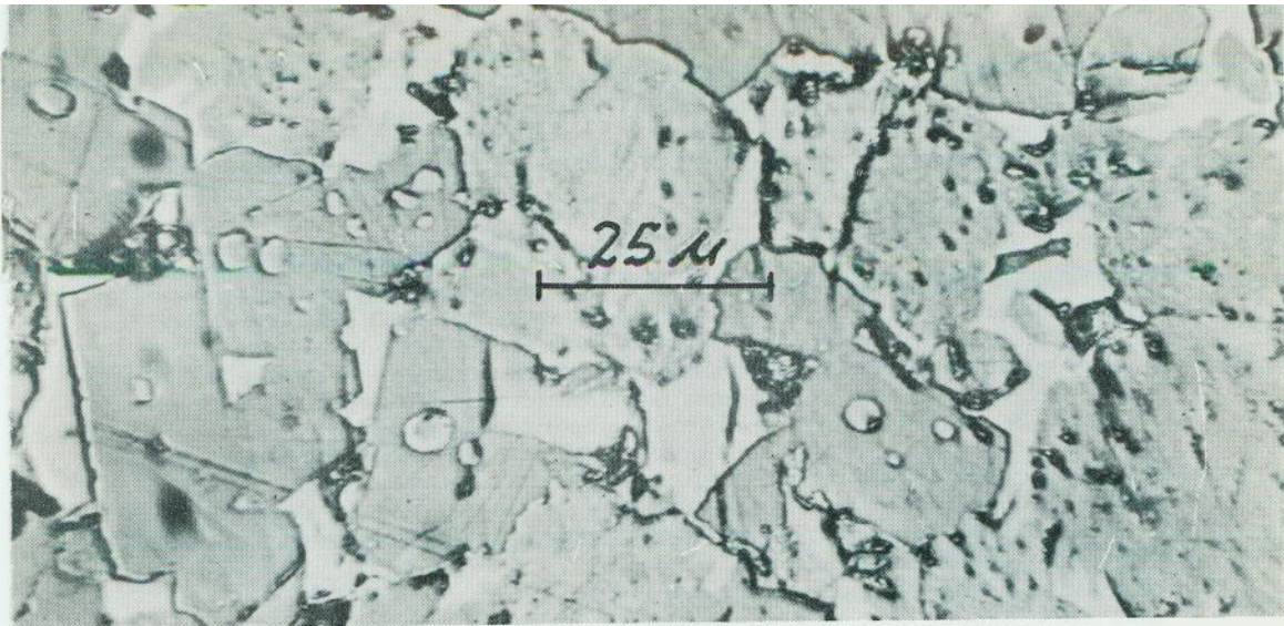
Fig. 4—Portland Cement Clinker as Seen in Polished Section, Etched with Distilled Water. Type II Composition. Angular, Gray Crystals Are C_3S . Rounded, Speckled Areas Are C_2S . Silver-White Interstitial Is C_4AF . Occasional Dark Interstitial Is C_3A .
