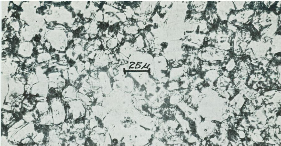
Fig. 1—Portland Cement Clinker as Seen in Thin Section Prepared with Hyrax Resin, Refractive Index 1.71. Type II Composition.
