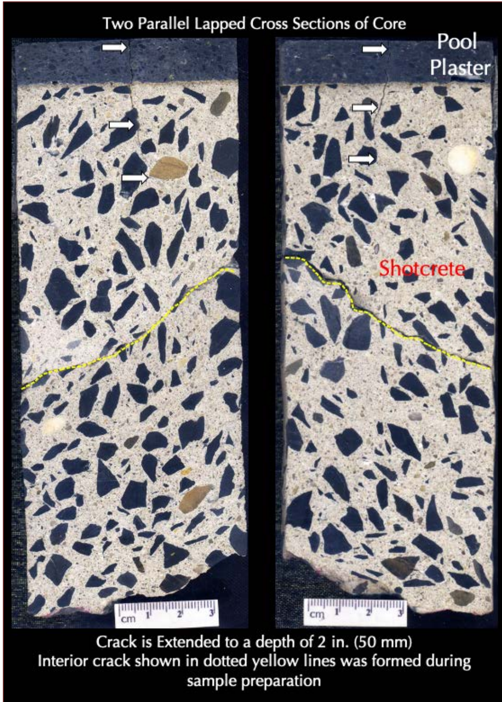
Figure 8: Lapped cross sections of Core No. 2 sectioned parallel to each other showing:
