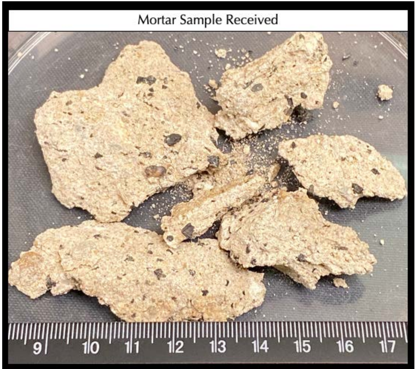
Figure 2: Mortar fragments received from the Church show an overall fragmented nature although individual pieces are relatively intact and do not break down into powders as many historic mortars when pressed with fingers. Sand contains a few dark particles that are scattered throughout the pieces. All fragments are uniform in medium gray to beige color tones and appeared to have no contamination from any other different mortar types. Therefore, all fragments were used for laboratory studies without a need for separation of any suspected contaminants.
