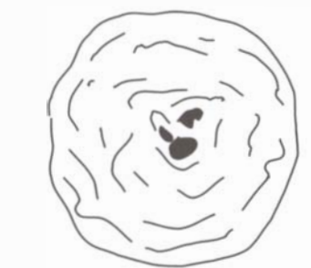
Uniform film layer, sometimes thicker at the edges
