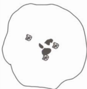
Dried puddles of solute that may appear shriveled and may exist in addition to a ring
