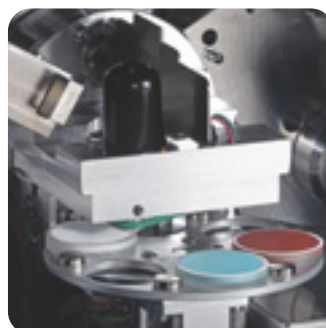
Six position sample changer
