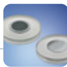
Low background holders for small sample amounts
