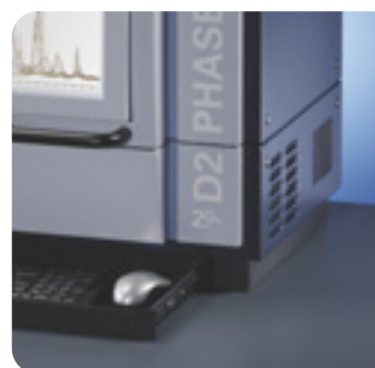
Integrated drawer for keyboard and mouse
