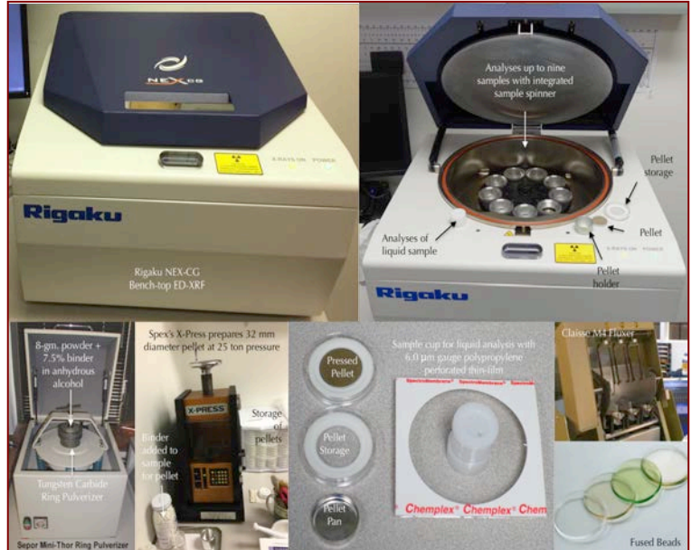
Fig. A8: Rigaku NEX-CG in CMC, which can perform analyses of 9 pressed pellet or fused bead of sample. Samples are prepared either as pressed pellet (usually the one already prepared for XRD) or can also accommodate fused bead with proper calibration of standard beads
