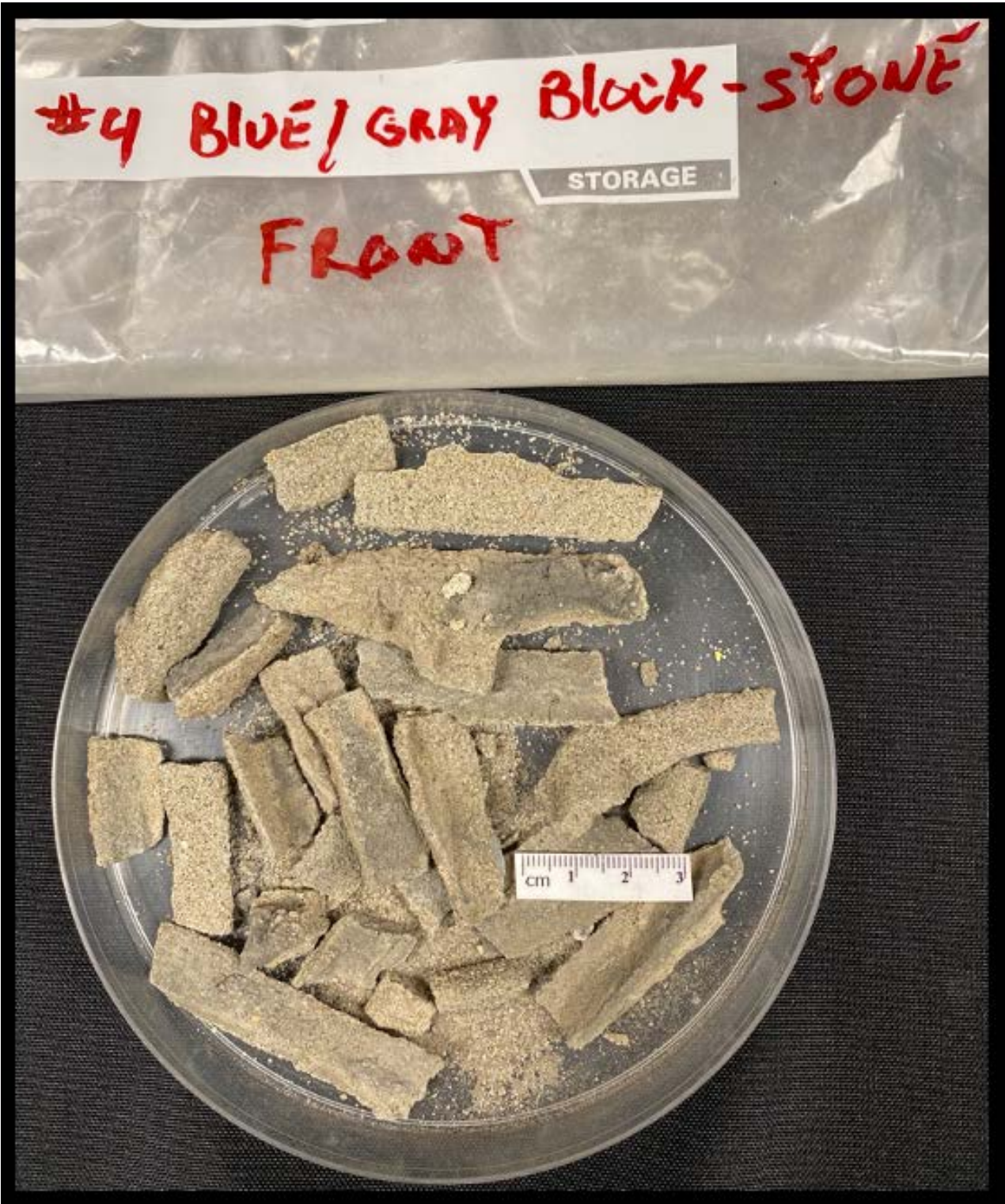
Figure 4: Mortar fragments #4 marked as 'Blue-Gray Black Stone Front' (hereafter described throughout the report as Mortar #4). The sample consists of numerous elongated pieces from the mortar joint that are mostly weathered brown to dark gray with sand-textured exposed faces. Overall integrity of the pieces are hard, in fact noticeably harder than typical historic lime mortar suggesting the potential presence of a Portland cement based component in the binder, which is responsible for the dense, hard, medium gray nature of fresh fractured surfaces of pieces.
