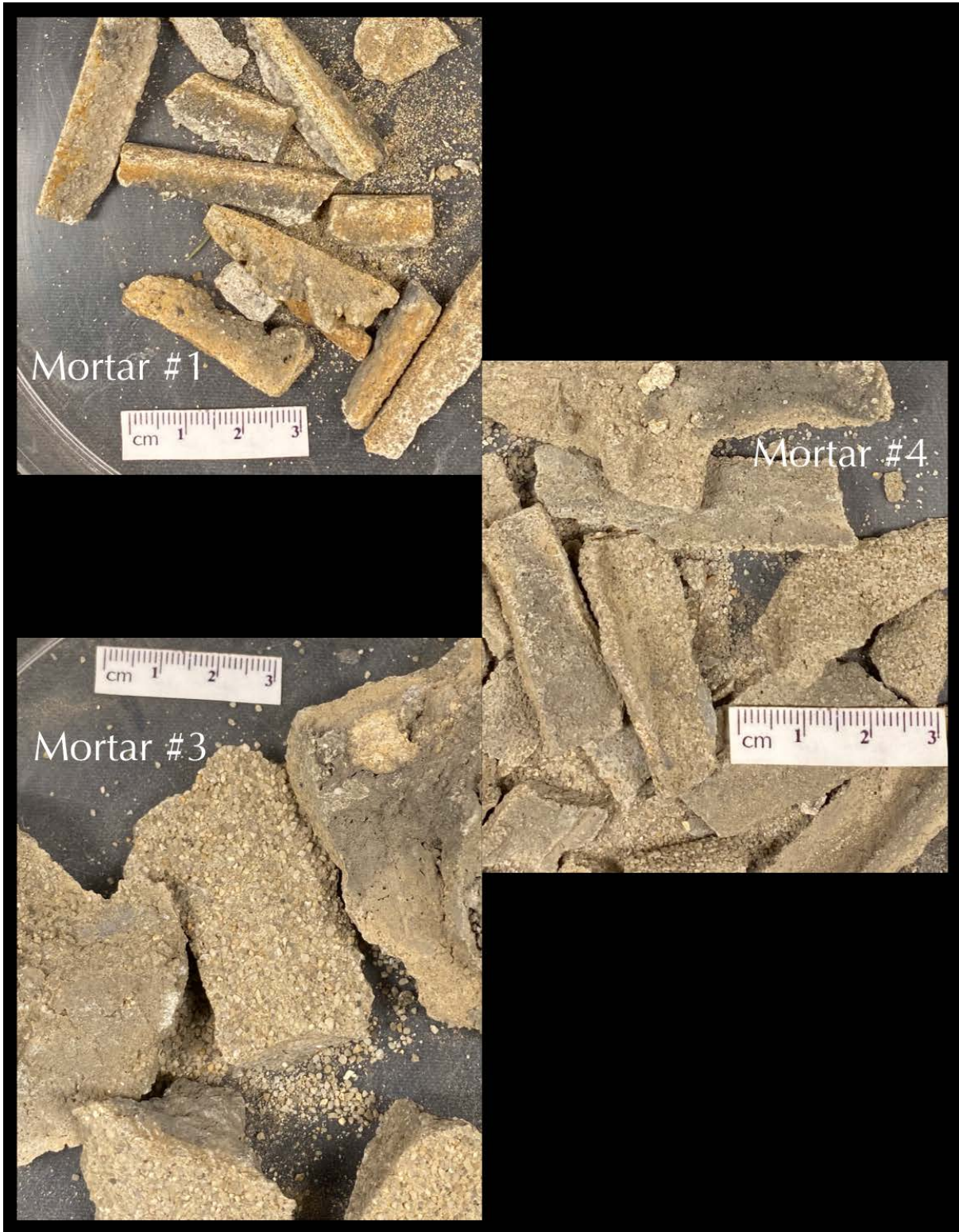
Figure 5: Comparison of three mortar samples received all showing more or less similar medium gray, dense, hard, sand-textured appearances indicating potential presence of similar binder and sand components in the samples. Grain size, shape, and gradation (sorting) of sand particles, however, appeared to differ from sample-to-sample indicating their derivation from different sources and/or times.
