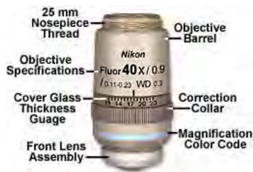
FIGURE 6.16: Nikon ultraviolet fluorite objective
