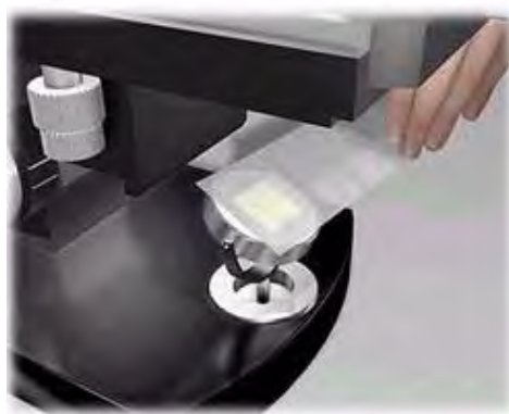
FIGURE 5.9: Centering an external lamp
