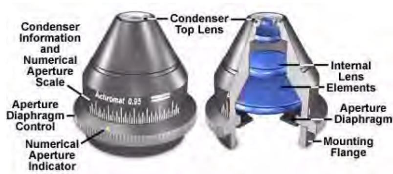
FIGURE 8.3: Achromatic condenser (NA=0.95)
