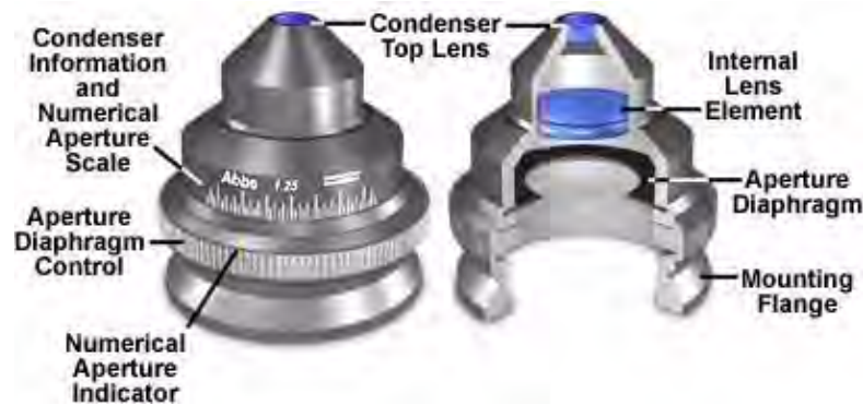
FIGURE 8.2: Abbe condenser (NA=1.25)
