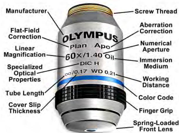
Figure 9. Specifications engraved on the barrel of a typical microscope objective. These include the manufacturer, correction levels, magnification, numerical aperture, immersion requirements, tube length, working distance, and specialized optical properties.
