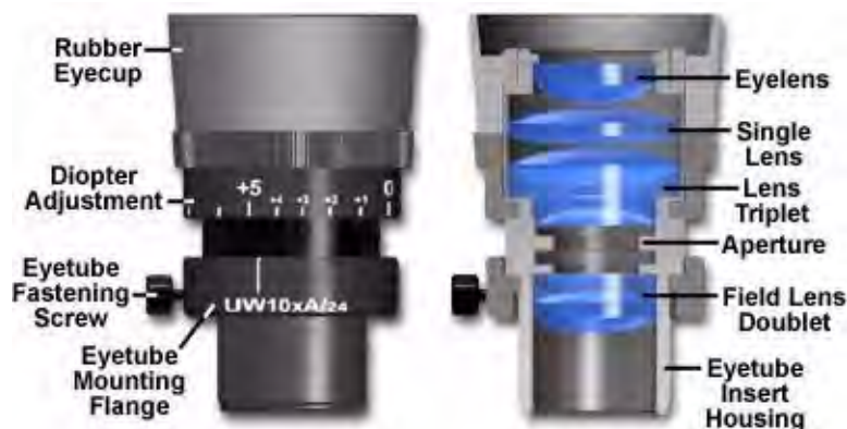
FIGURE 7.1: Aberration-free 10x eyepiece with dioptric adjustment
