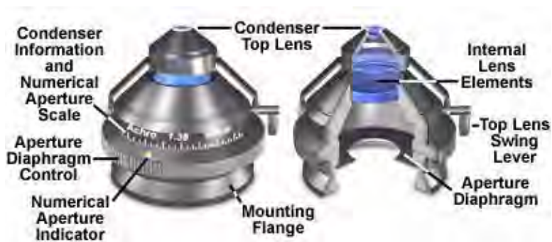
FIGURE 23.14: Swing-out top lens condenser (NA=1.35)
