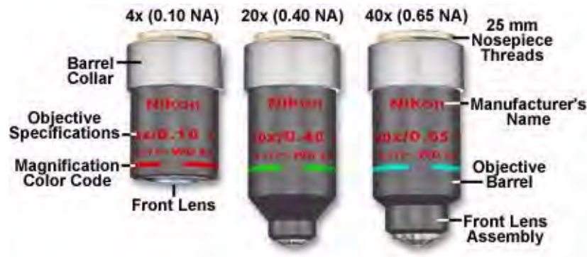
FIGURE 6.15: Polarized light objective color codes
