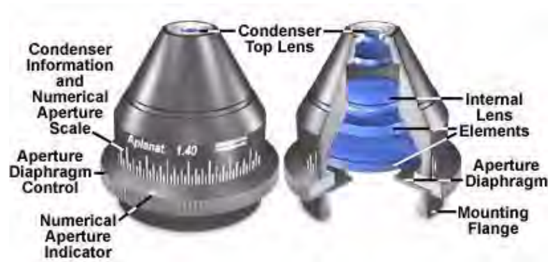
FIGURE 8.4: Aplanatic condenser (NA=1.4)
