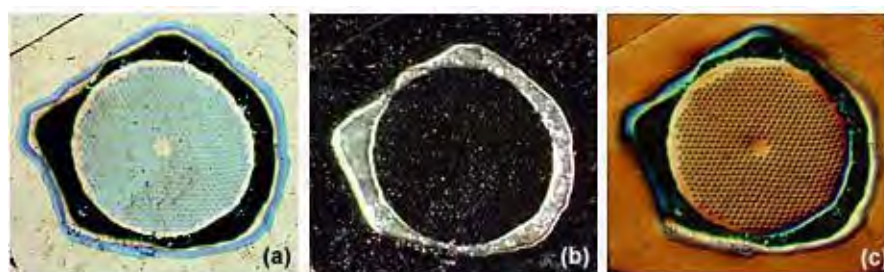
FIGURE 19.12: Niobium—TiN superconducting filament in copper matrix
