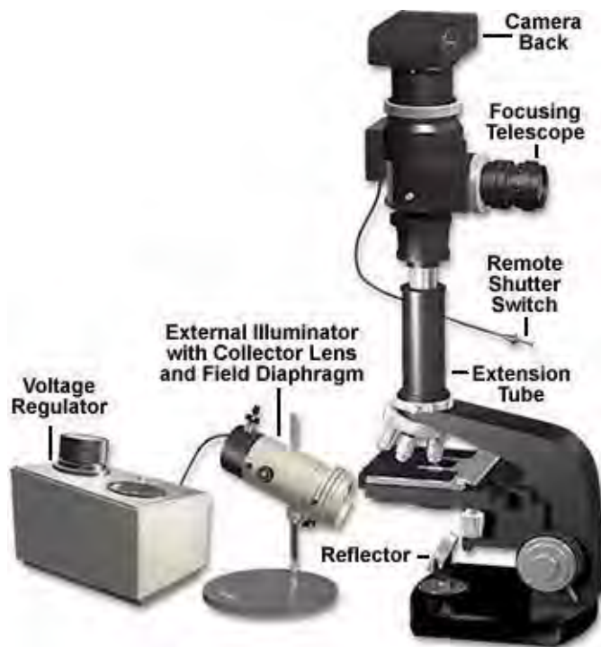
FIGURE 5.6: Transmitted light microscope with external lamp and camera attachment
