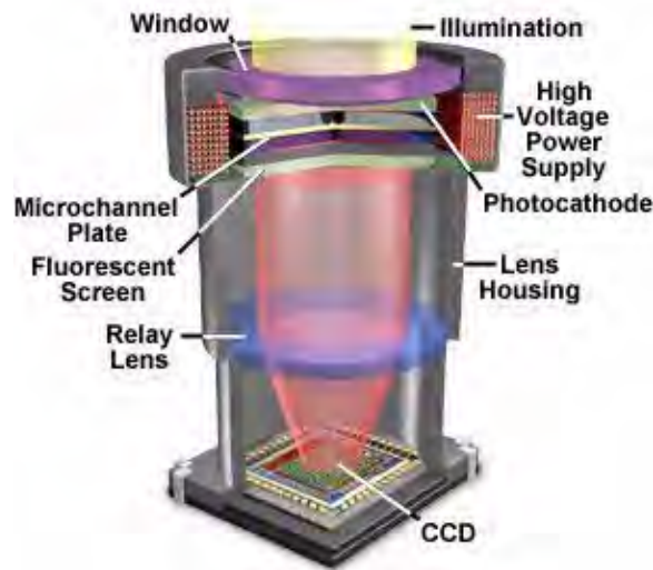
FIGURE 28.7: Image intensifier with Relay lens
