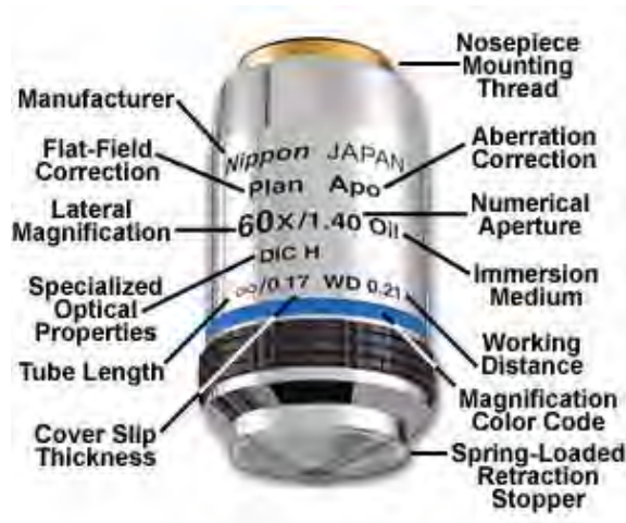
FIGURE 6.9: 60x plan apochromat objective
