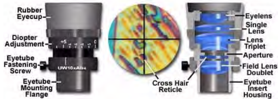
FIGURE 23.19: 10x eyepiece with diometer adjustment and cross hair reticle
