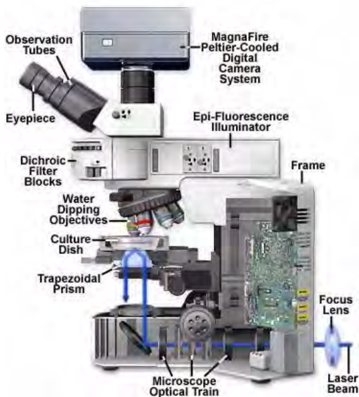
FIGURE 17.14: Upright microscope TIR configuration
