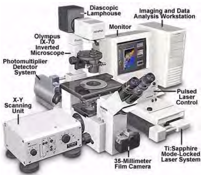
FIGURE 16.1: Multiphoton excitation fluorescence microscope configuration
