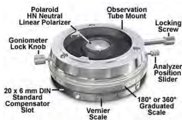
FIGURE 23.13: Analyzer intermediate tube
