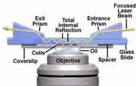
FIGURE 17.12: Substrate/prism inverted TIRF configuration
