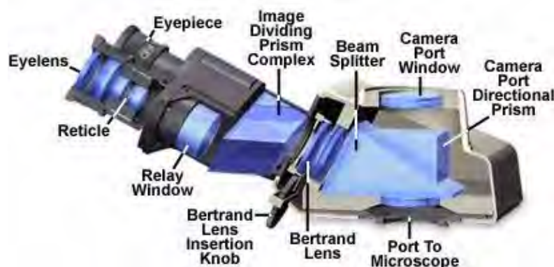
FIGURE 23.18: Binocular microscope observation tube with Bertrand Lens
