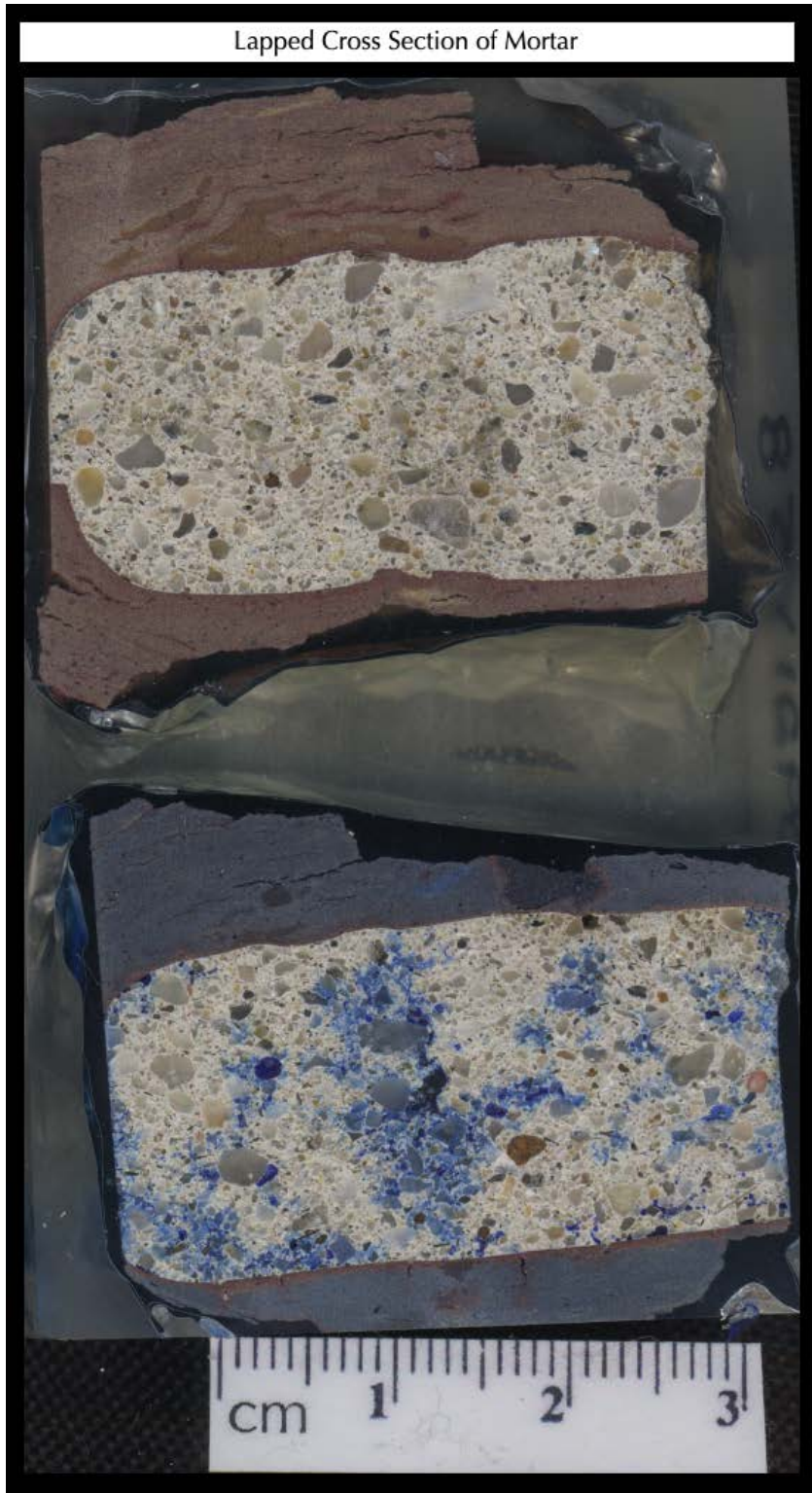
Figure 11: Lapped cross section of two pieces of mortar after encapsulating in a low-viscosity epoxy. The top piece was encapsulated in a clear epoxy medium, whereas the bottom piece was encapsulated with a blue dye-mixed epoxy to highlight cracks voids and pore spaces in mortar in thin section. A thin section was subsequently prepared from this polished epoxy-encapsulated block.
