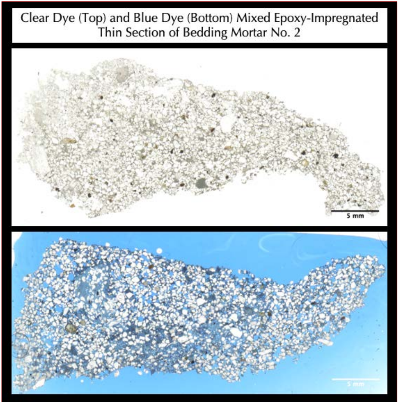
Figure 16: Clear epoxy (top) and blue dye-mixed epoxy (bottom) impregnated thin section of mortar fragment from the bedding mortar No. 2 taken by using a flatbed film scanner, where thin section was placed on a scanner with a polarizing filter to recreate plane polarized light view of sample to show the sand grain size, shape, angularity, and distribution, and pore and void spaces in mortar from blue epoxy.
