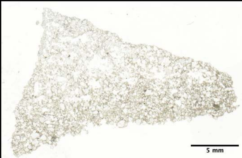
Figure 18: Clear epoxy (top) and blue dye-mixed epoxy (bottom) impregnated thin section of mortar fragment from the pointing mortar No. 3 taken by using a flatbed film scanner, where thin section was placed on a scanner with a polarizing filter to recreate plane polarized light view of sample to show the sand grain size, shape, angularity, and distribution, and, pore and void spaces in mortar from blue epoxy.
