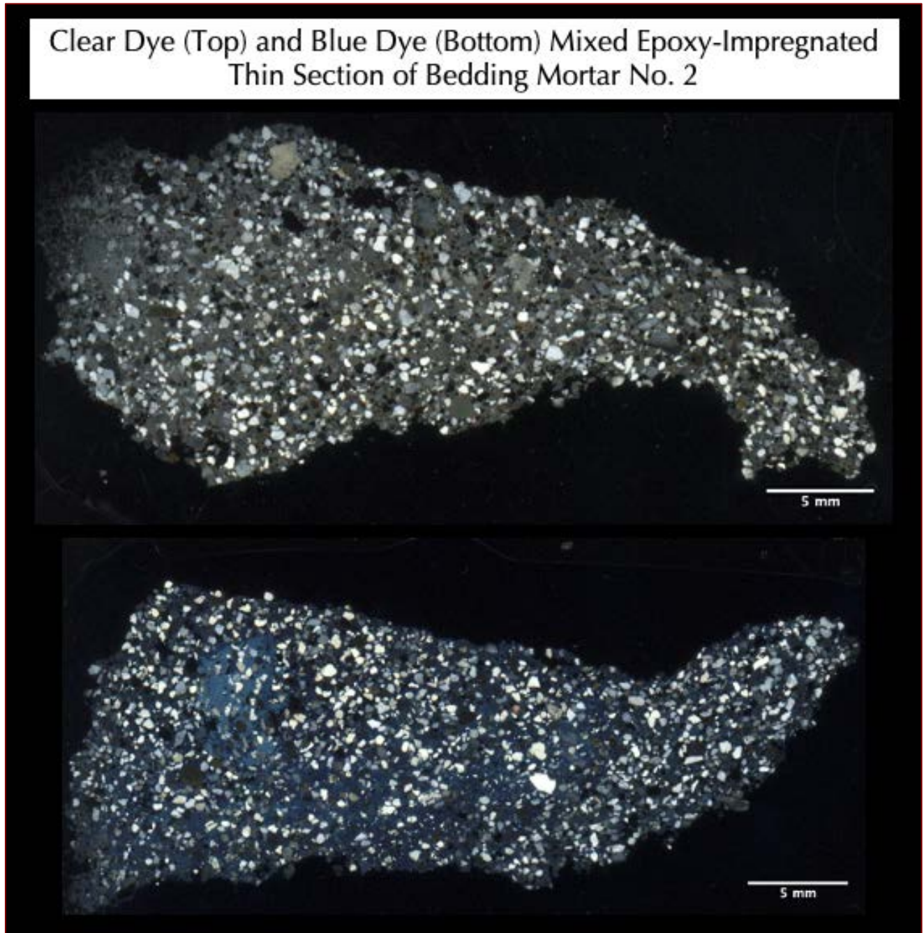
Figure 17: Clear epoxy (top) and blue dye-mixed epoxy (bottom) impregnated thin section of mortar fragment from the bedding mortar No. 2 taken by using a flatbed film scanner, where thin section was placed on a scanner with two perpendicular polarizing filters to recreate cross polarized light view of sample to show the siliceous composition of sand and variably carbonated paste.
