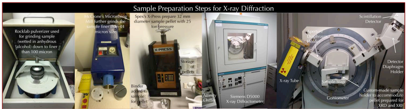
Fig. A7: Siemens D5000 X-ray diffractometer and MDI Jade search/match software used for determination of mineralogical composition of mortar. Left to right: Rocklab pulverizer for initial grinding of sample with anhydrous alcohol; McCrone micronizing mill for final grinding; Spex 25-ton press for pellet preparation; Siemens D5000 X-ray diffractometer; and custom-made sample holder to place a 32-mm diameter pellet on sample stage.
