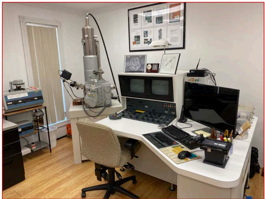
Fig. A3: Camscan SEM equipped with Ametek EDAX silicon drift detector for elemental analyses, secondary electron detector for morphological analyses and high-resolution YAG backscatter electron detector for microstructural analyses, and 4Pi revolution module for data collection and analyses.
