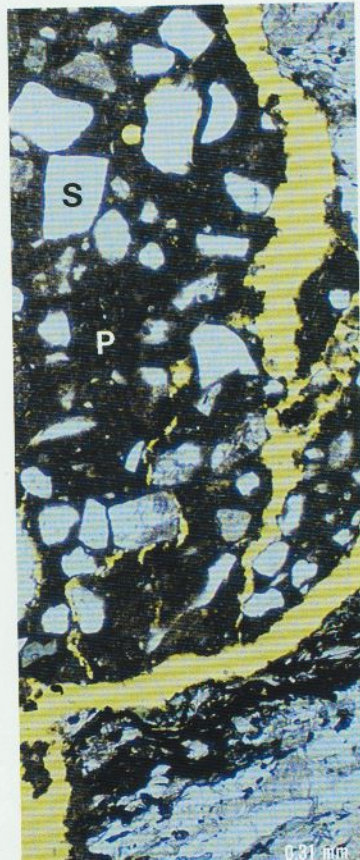
Figure 18. 25X. Wide, very irregular cracks, presumably
