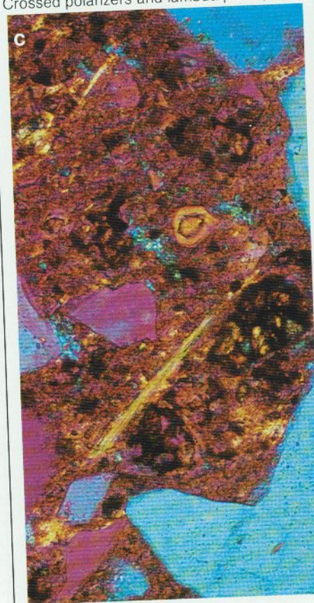
Figure 6. Magnification 63X with polarization microscope. The same motive shown in 4 (b) with unhydrated cement (P) with unhydrated
