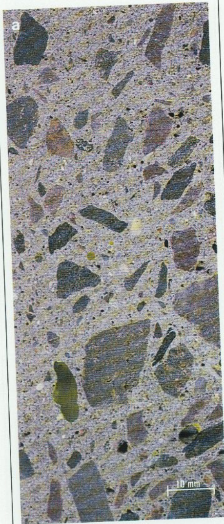
Figure 2 A cut section makes it possible to examine the coarse aggregate, compaction, large cracks etc.
