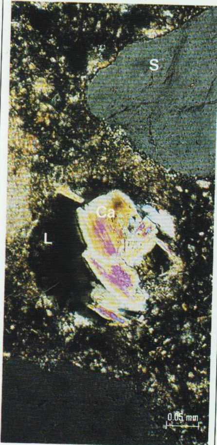
Figur 13. 160X. Void (L) partly filled with coarse calcium hydroxide crystals (Ca). Small calcium hydroxide crystals are seen in the surrounding paste. Crossed polarizers.
