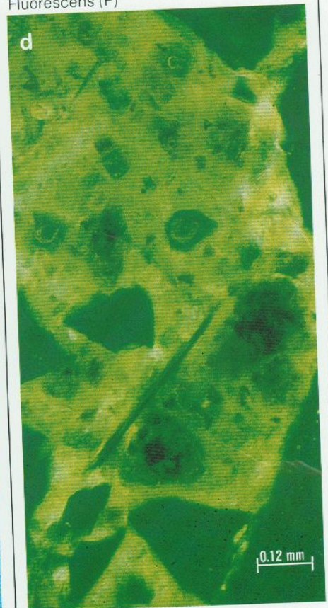
Figure 6. Magnification 63X with polarization microscope. The same motive shown in 4 (b) with unhydrated cement (P) with unhydrated
