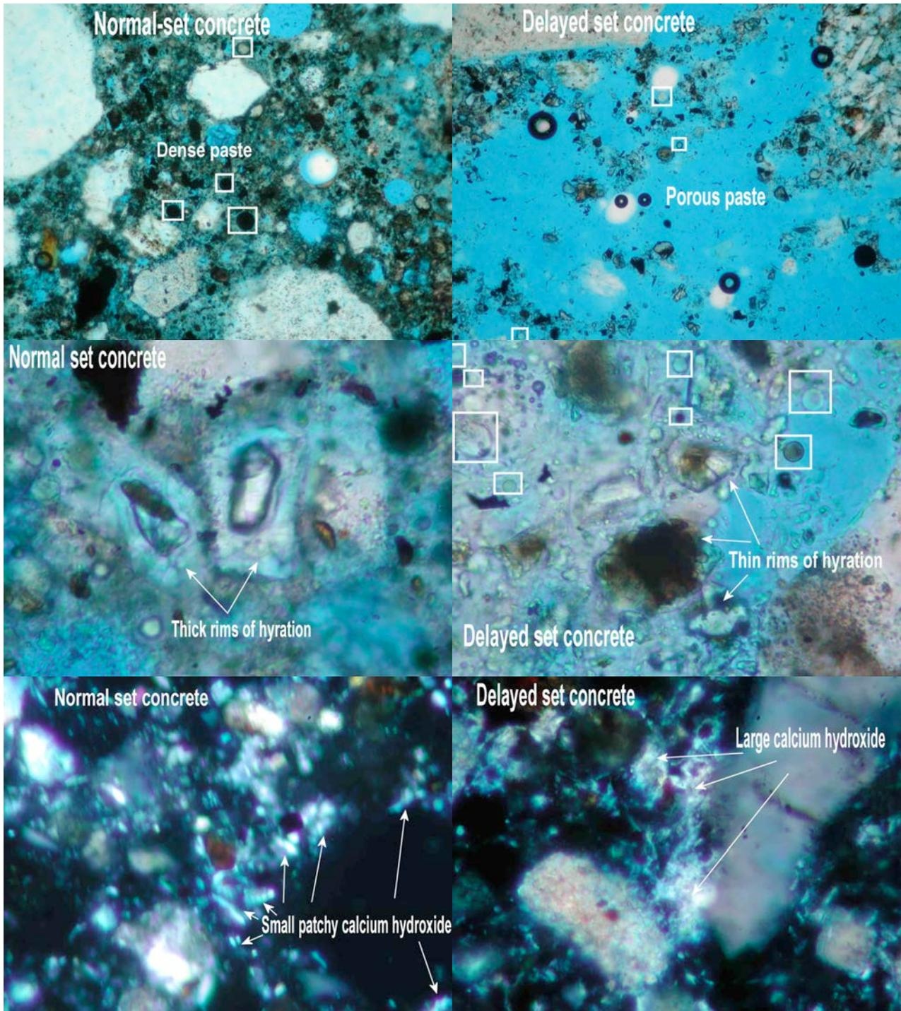
**Figure 4:** Microstructural differences between the normal and delayed set concretes: Top - Difference in porosities of the paste (fly ash particles are boxed; Middle – Difference in degrees of cement hydration; Bottom – Difference in sizes of calcium hydroxide component of portland cement hydration. Some fly ash particles in the paste are boxed. Field widths are 0.5 mm.
