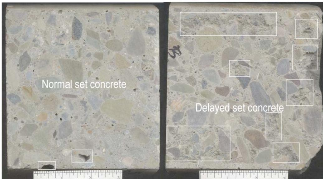
**Figure 3:** Cross-sections of portions of cylinders of normal and delayed set concretes showing: (a) crushed gravel coarse aggregates; (b) the distribution and overall poor grading of the aggregates; and (c) the loss of paste (boxed) during sectioning in the delayed set concrete. The scales are in 1-in. numerical increments.
