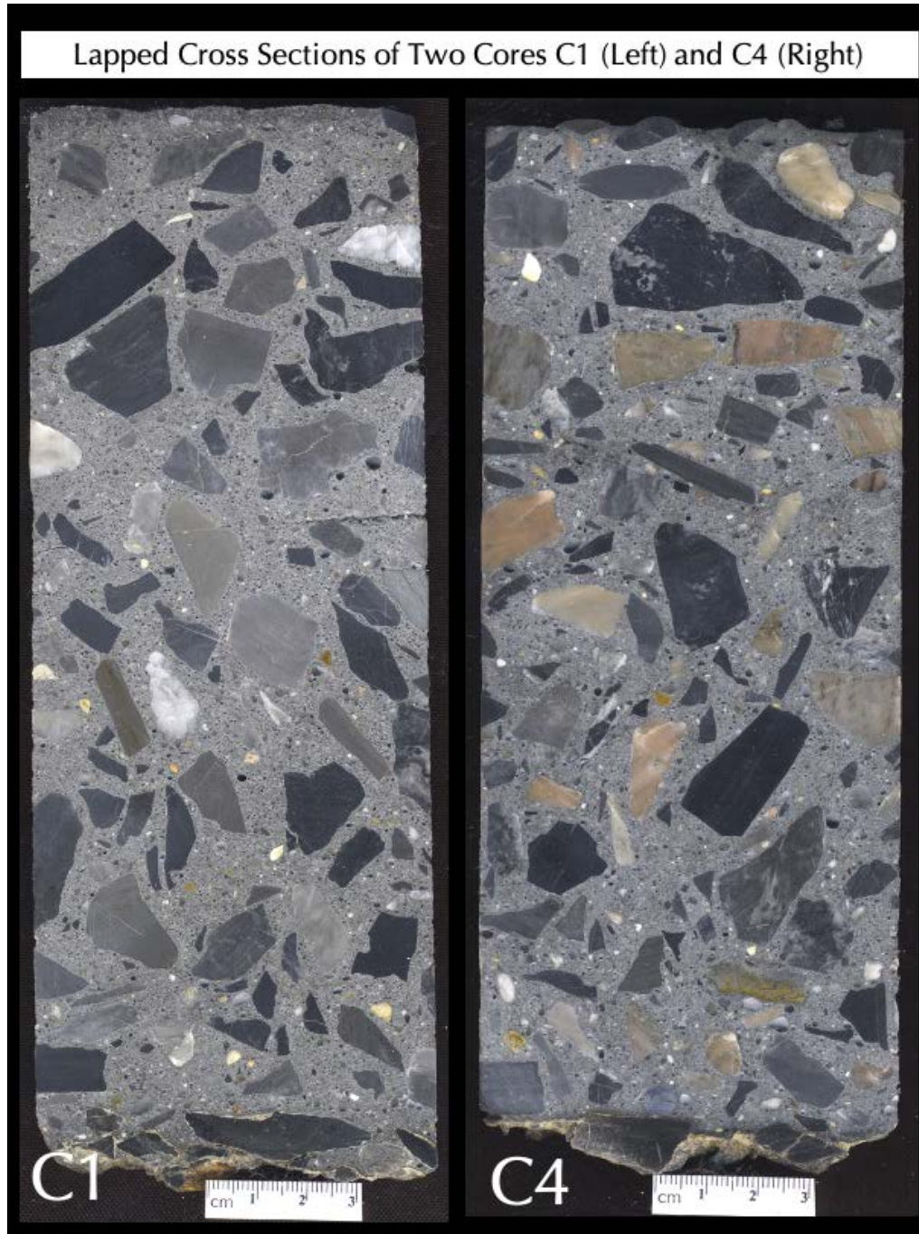
Figure 13: Lapped cross sections of Cores C1 and C4 showing overall densified concrete containing compositionally similar, medium to dark gray, angular, equidimensional to a few elongated, well-graded, well-distributed, crushed limestone coarse aggregates, dark gray paste due to the incorporation of fly ash along with Portland cement, rough exposed surface ends at top, and, adhered subbase material at the bottom ends indicating full-depth recovery of cores from the slab. Notice the overall good consolidation of concrete at both core locations as well as sound, visually crack-free natures, and free of any discolorations at the surface regions from any surface contaminants.
