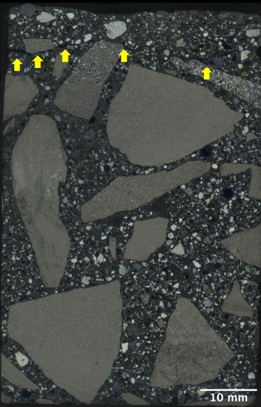
Figure 33: Blue dye-mixed epoxy-encapsulated thin section of Core C1 taken by using a flatbed film scanner, where thin section was scanned with two polarizing filters at perpendicular orientations to recreate cross polarized light view of sample where crushed limestone coarse aggregate and natural siliceous sand fine aggregates are highlighted. Arrows show near-surface incipient delamination.
