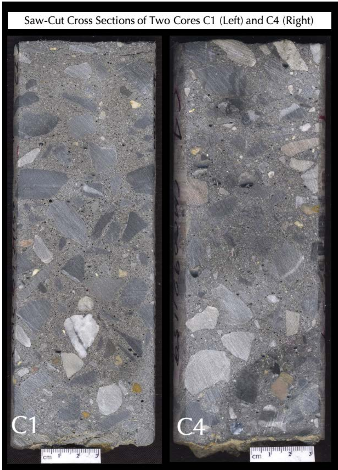
Figure 14: Saw-cut cross sections of Cores C1 and C4 showing overall densified concrete containing compositionally similar, medium to dark gray, angular, equidimensional to a few elongated, well-graded, well-distributed, crushed limestone coarse aggregates, dark gray paste due to the incorporation of fly ash along with Portland cement, rough exposed surface ends at top, and adhered subbase material at the bottom ends indicating full-depth recovery of cores from the slab.
