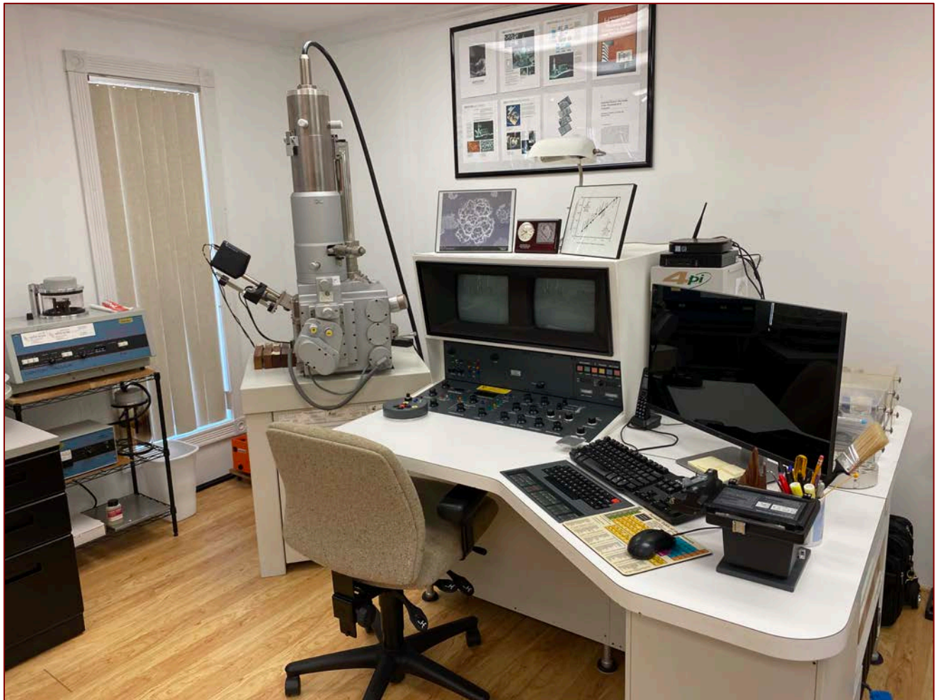
Figure 9: SEM-EDS: Cambridge CamScan Series II Scanning Electron Microscope and 4Pi Revolution software, backscatter detector, secondary electron detector, and energy-dispersive X-ray fluorescence spectrometer used for microstructural and microchemical analyses of surface deposits in Core C1 as well as of the ash sample.
