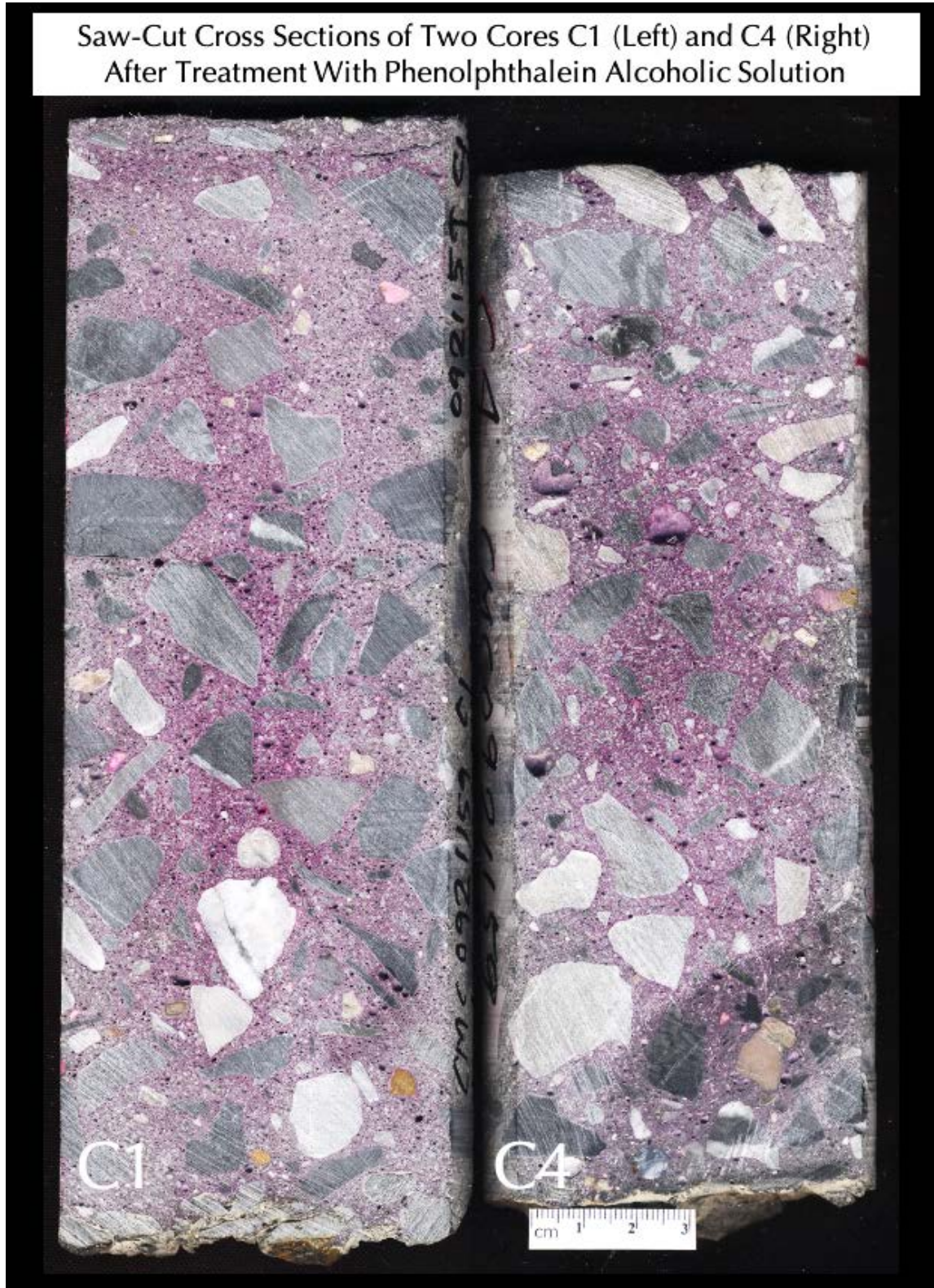
Figure 15: Saw-cut cross sections from Figure 14 after treatment with phenolphthalein alcoholic solutions showing overall dense non-carbonated nature of concrete except only minimal patchy carbonation at the surface that are only detected from thin sections.
