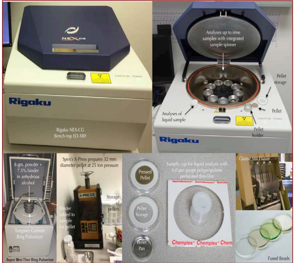
Figure 11: Rigaku NEX-CG in CMC, which can perform analyses of 9 pressed pellet or fused bead of sample. Samples are prepared either as pressed pellet (usually the one already prepared for XRD) or can also accommodate fused bead with proper calibration of standard beads.
