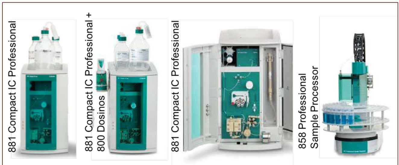
Figure 12: Set-ups for chloride and sulfate analysis by ion chromatography and pH of ash sample.
