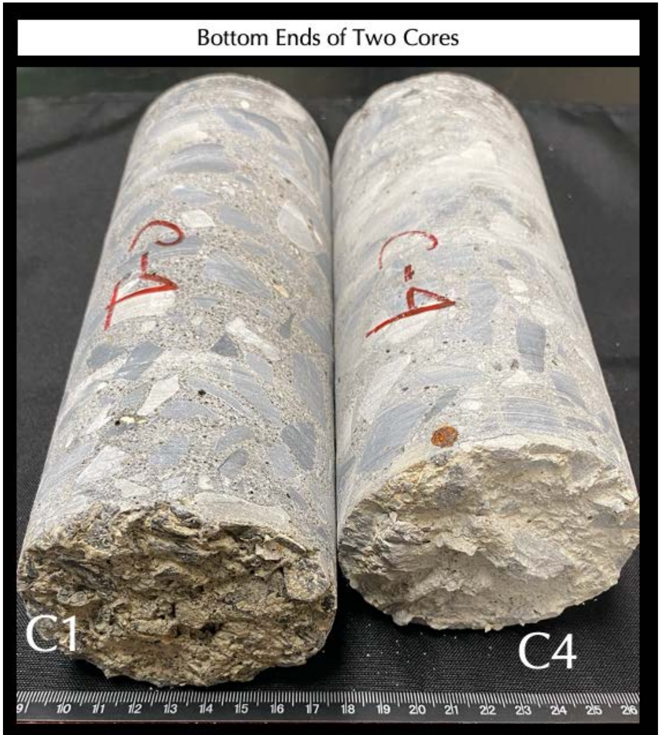
Figure 7: Opposite bottom ends of the cores, as received, showing the subbase materials indicating full-depth retrieval of cores at their respective locations.
