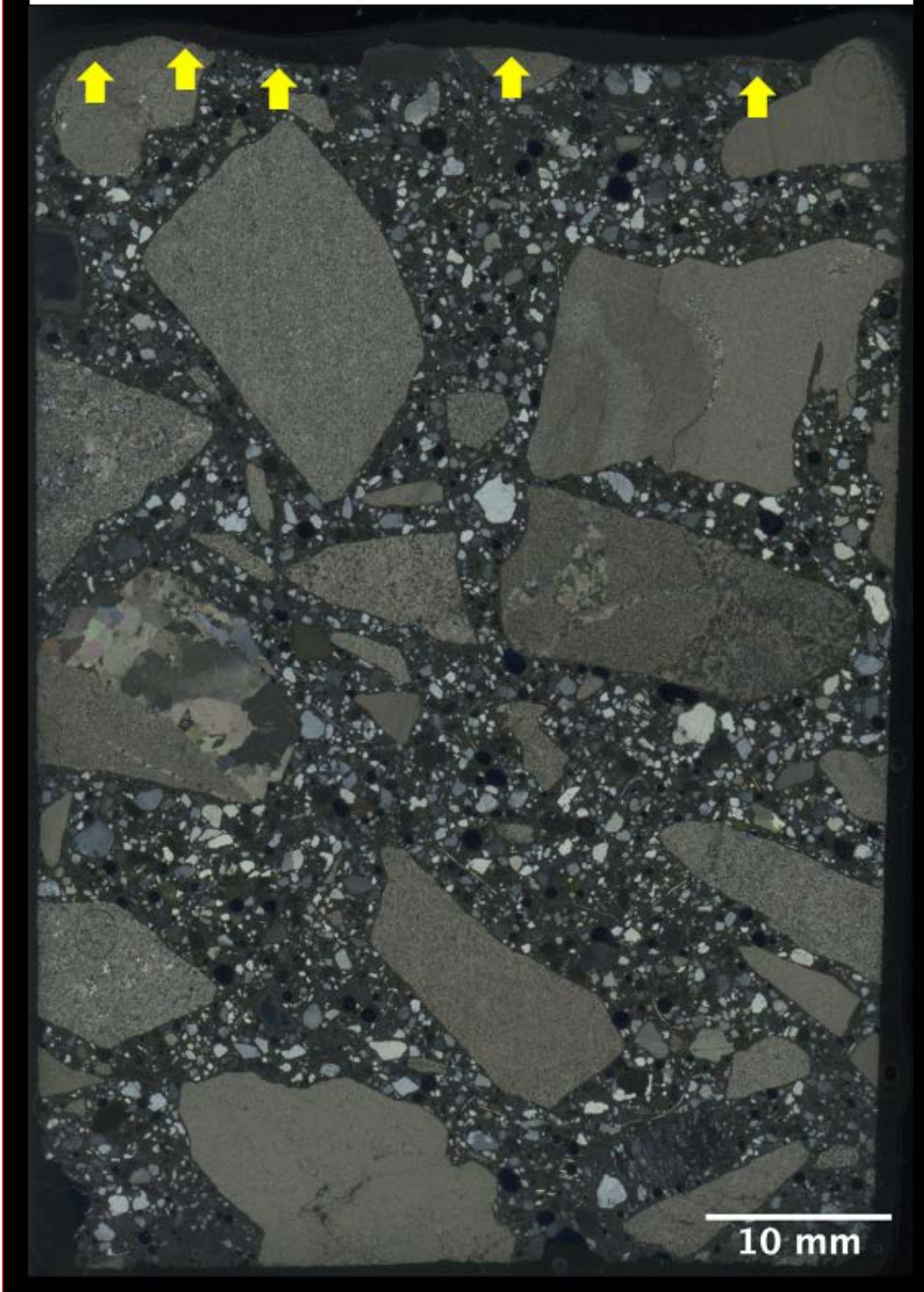
Figure 35: Blue dye-mixed epoxy-encapsulated thin section of Core C4 taken by using a flatbed film scanner, where thin section was scanned with two polarizing filters at perpendicular orientations to recreate cross polarized light view of sample where crushed limestone coarse aggregate and natural siliceous sand fine aggregates are highlighted. Arrows show surface delamination.
