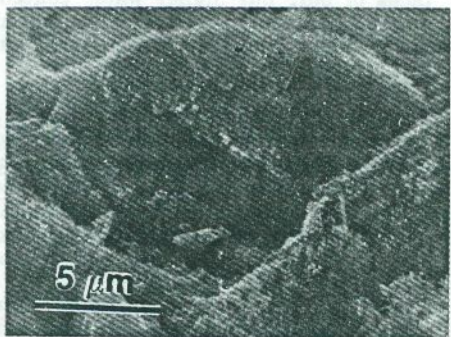
Fig. 6. An "inner" hydration product cement grain residue showing dense Type IV morphology.
