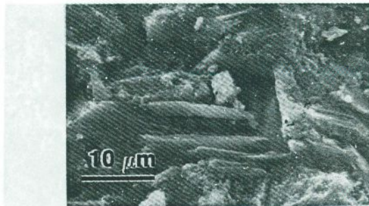
Fig. 8. Typical intermingling of layered calcium hydroxide with Type III C-S-H gel.
