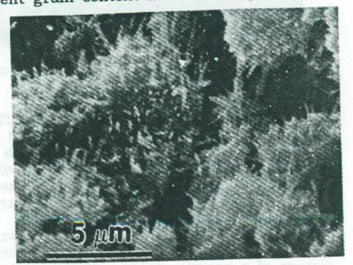
Fig. 3. Type I C-S-H gel particles growing radially around cement grains.
