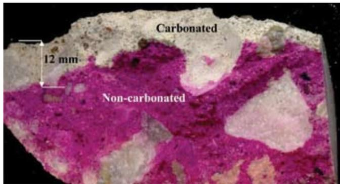
Fig. 2: Depth of carbonation of a freshly fractured surface determined by spraying with a phenolphthalein solution that turns pink at noncarbonated areas
