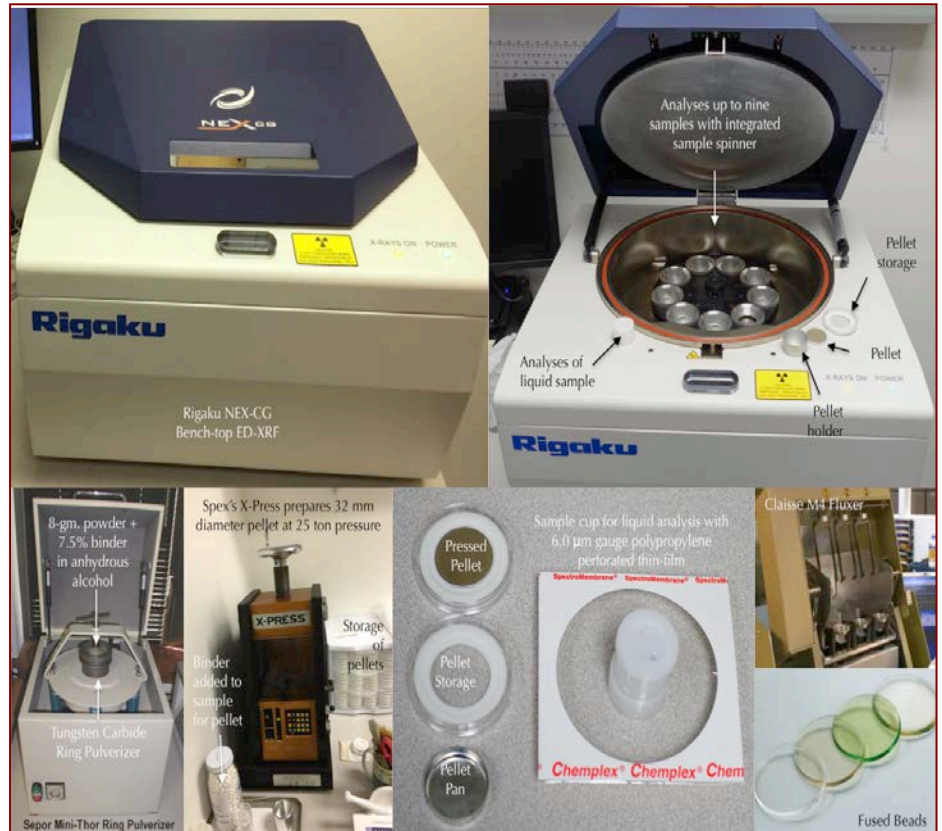
Figure 2: Rigaku NEX-CG in CMC, which can perform analyses of 9 pressed pellet or fused bead of sample. Soil samples are prepared as pressed pellets.
