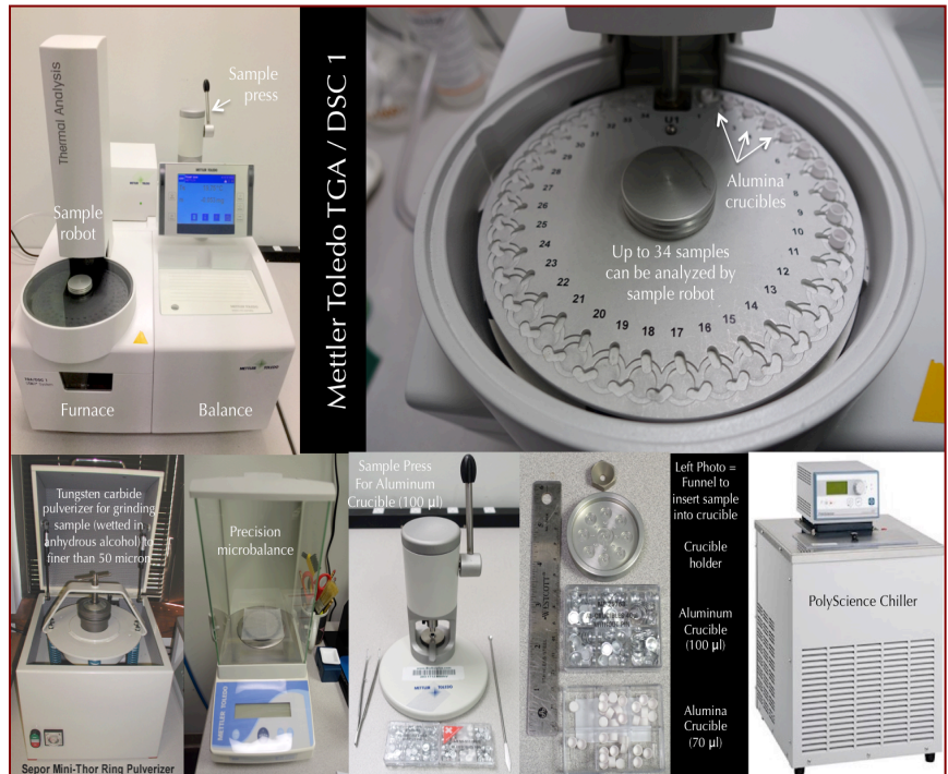
Figure 2: Mettler-Toledo simultaneous TGA/DSC1 unit in CMC that can accommodate 32 samples. The top left photo shows the TGA/DSC1 unit with sample robot for automation as well as the sample holder for pressing aluminum sample holders. Sample is pulverized in a ring pulverizer shown in the bottom left, then a small amount (usually 30-70 mg) is weighed in a precision balance (shown 2 nd from left in bottom row) and taken in an alumina sample holder (without lid). For DSC measurements up to 600°C, sometimes sample is taken in an aluminum holder and pressed in sample press (3 rd from left in bottom row) and pierced with a needle for release of volatiles from decomposition. A PolyScience chiller (rightmost one in the bottom row) is used to cool the furnace. An ultrapure nitrogen gas is purged through the system during analyses.
