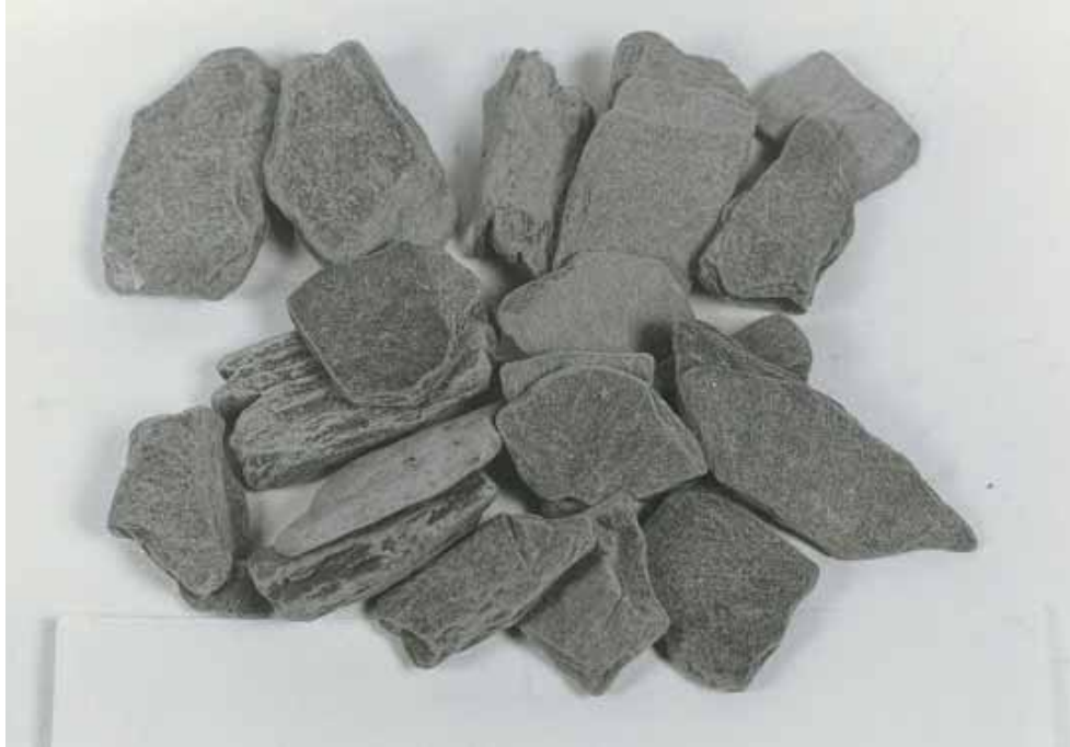
Figure 206. Shaley particle shape of crushed slate aggregate.
