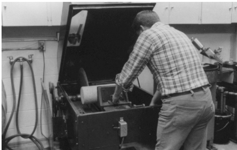
Figure 4. Large, oil-cooled, continuous diamond-edged rotary saw.
