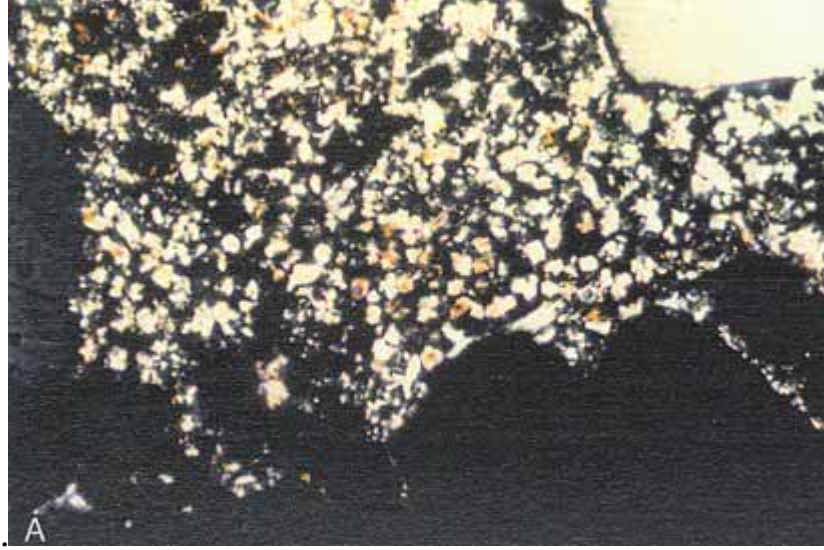
Figure 159. Thin section of interior portion of HCC: (A) Viewed with crossed nicols (bright area shows the high birefringence of the calcite of the carbonated area).
