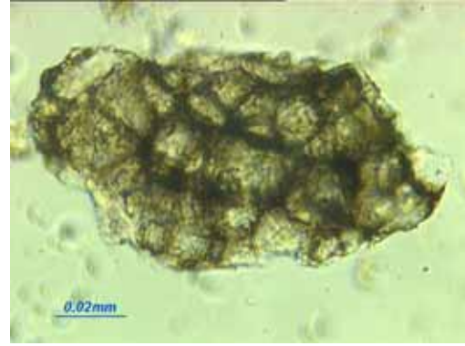
Figure 133. Immersion mount of belite cluster with darker interstitial aluminates and ferrite.
