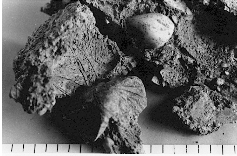
Figure 30. Fragments of concrete destroyed by freezing before final setting.
