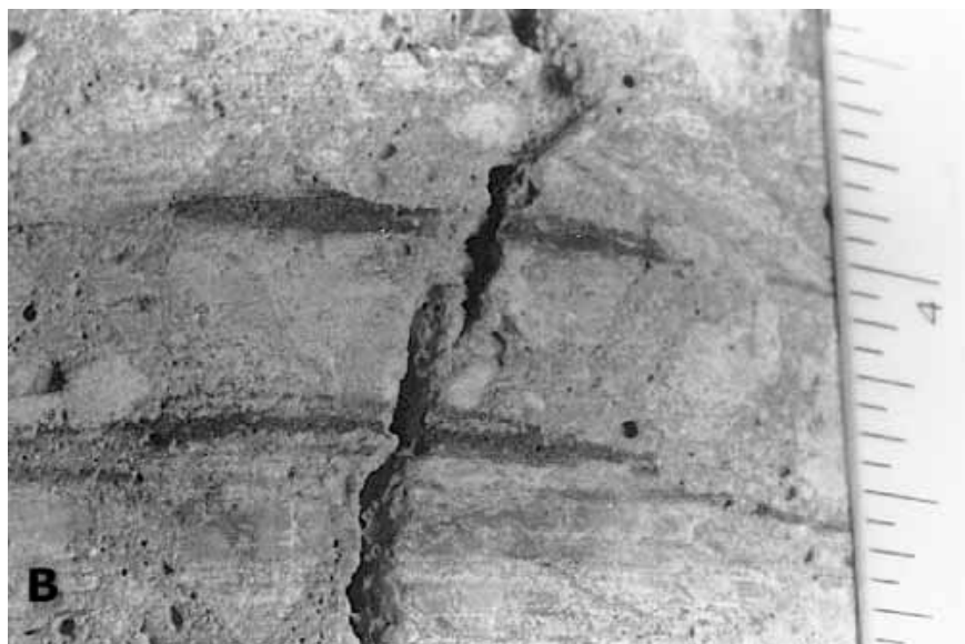
Figure 38. Bridge of paste across plastic shrinkage crack: Closeup of bridge.
