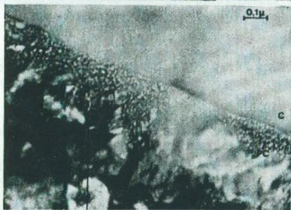
Fig. 38. Contact zone between calcite and cement paste, ion-beam-thinned section of a one-year-old sample. (Courtesy J-P Ollivier.)
