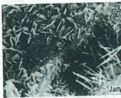
Fig. 17. Fracture surface of a 14-day-old paste. The edge of a hydrate shell runs diagonally across the micrograph. On the inner surface (top left) many plates of AFm can be seen. Outside the shell AFt rods protrude into the pore space. (Courtesy A. Ghose.)
