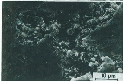
Fig. 39. Area of fracture surface in a one-day-old mortar, adjacent to an aggregate particle. Beyond the surface layer (some of which adhered to the aggregate during fracture) can be seen 'rosettes' of C-S-H from the hydration of small cement grains and long rods of Aft.
