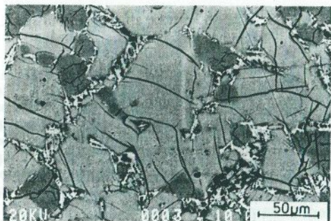
Fig. 1. Microstructure of a commercial clinker (bse image). Light-gray crystals of alite and darker rounded crystals of belite can be seen in a matrix of the interstitial phases—ferrite (light) and aluminate (darker). Porosity (black) can also be seen.
