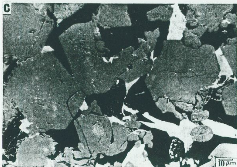
Fig. 2. (a)–(d). Optical micrographs of polished surfaces of normal Portland cement, illustrating the effects of chemical etching: (b) is of the same area as (a) but is shown after etching with 10% boric acid in water to bring out the silicate (light grey—C 2 S; dark grey—C 3 S) and interstitial (white) phases (the scale on (b) is the same as that on (a)); (c) and (d) show the result of 10% potassium hydroxide etch to
