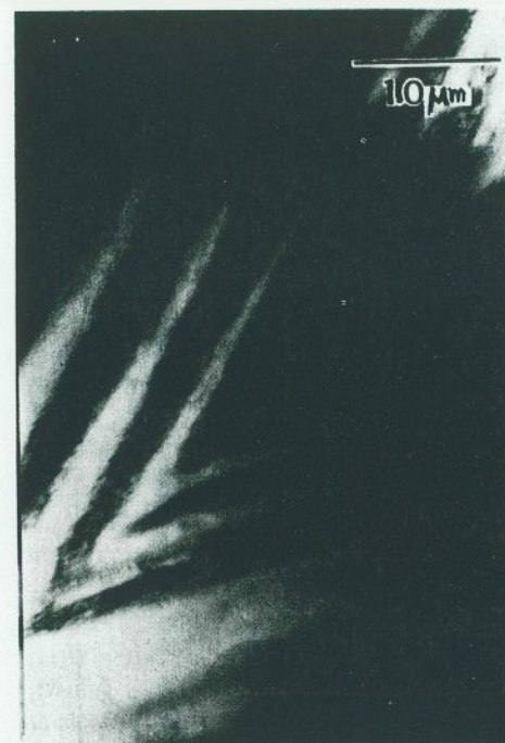
Fig. 18. TEM micrograph 154 of a Ba-stabilised \alpha' - C_2S grain showing precipitates in two sets of bands meeting at an angle of about 45°.
