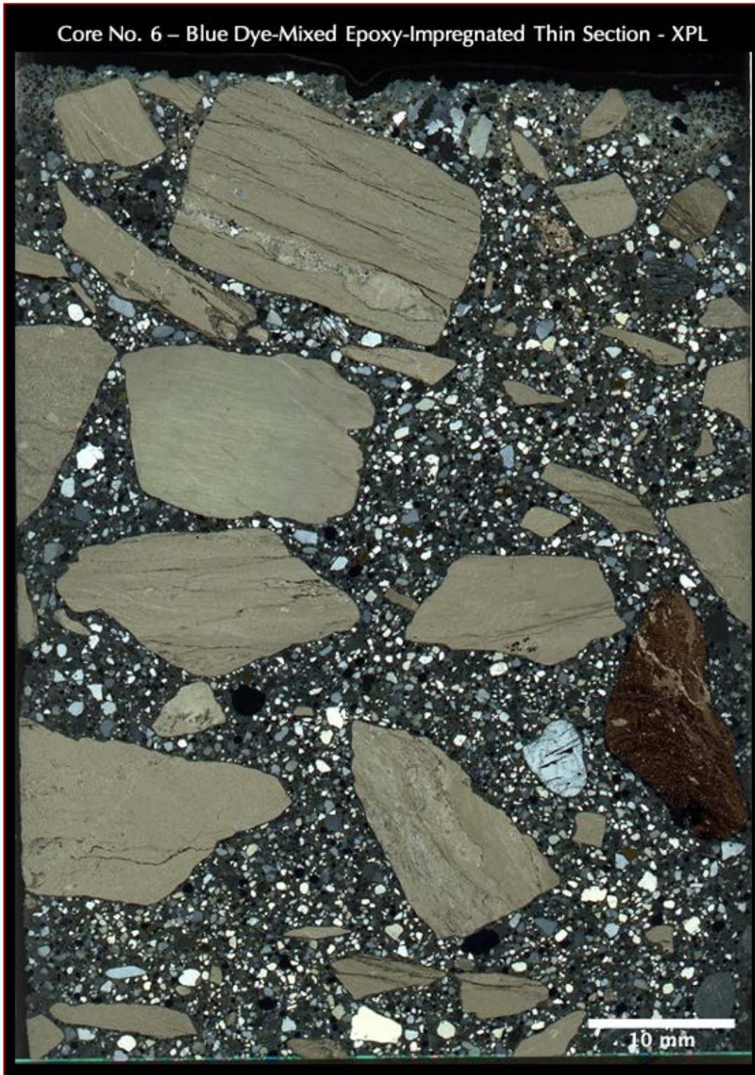
Figure 34: Blue dye-mixed epoxy-impregnated large-area (50 mm × 75 mm size) thin section of Core 6 shown in crossed-polarized light mode to highlight the coarse and fine aggregates in concrete. The thin section was scanned on a film scanner with two perpendicular polarizing filters.
