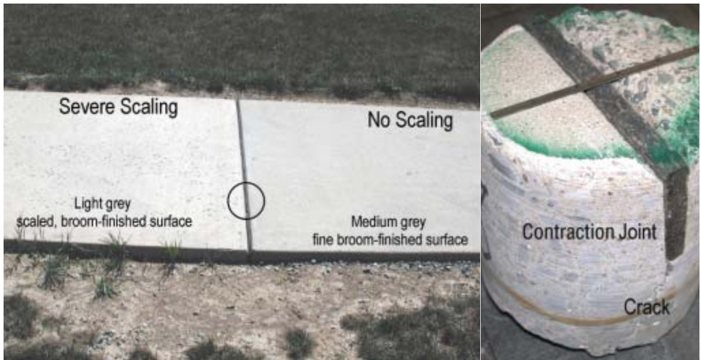
Fig. 2: Case study II (Scaling due to finishing in the presence of excess water at the surface)—Concrete core from a contraction joint showing adjacent sound and scaled surfaces
