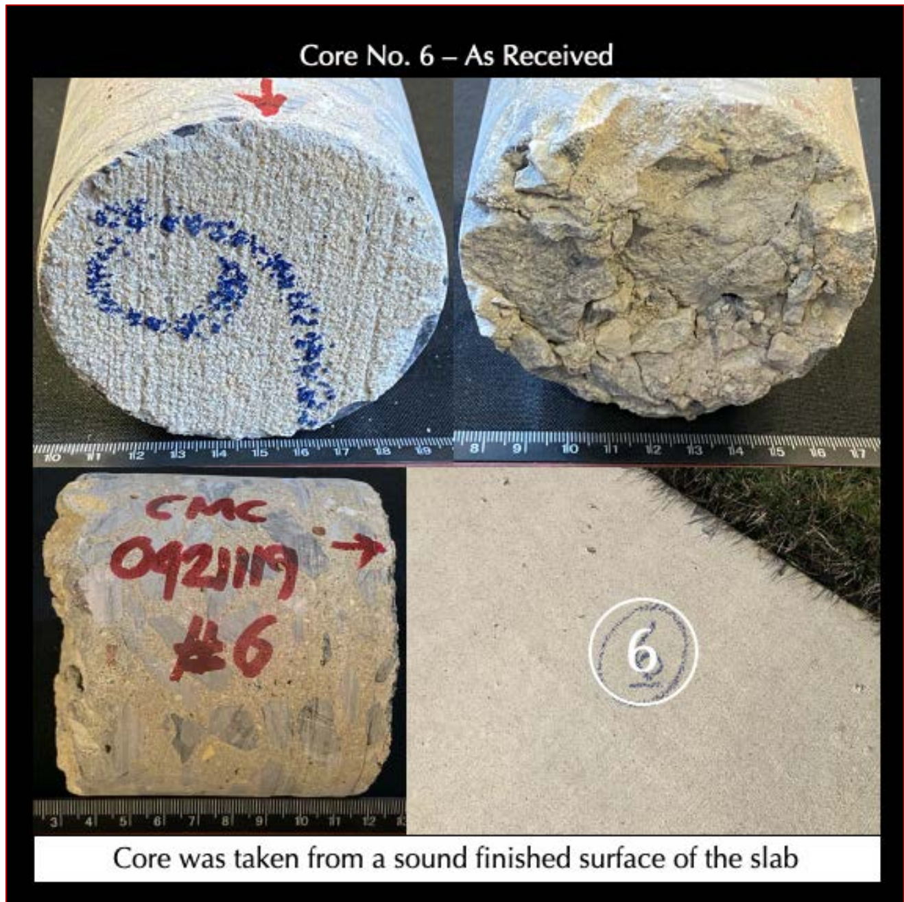
Figure 13: Core 6 as received showing the sound fine broom-finished surface, which is consistent with its collection from a sound location of slab as seen in the bottom right inset, bottom surface of core at the top right, and side cylindrical surface at the bottom left photo.
