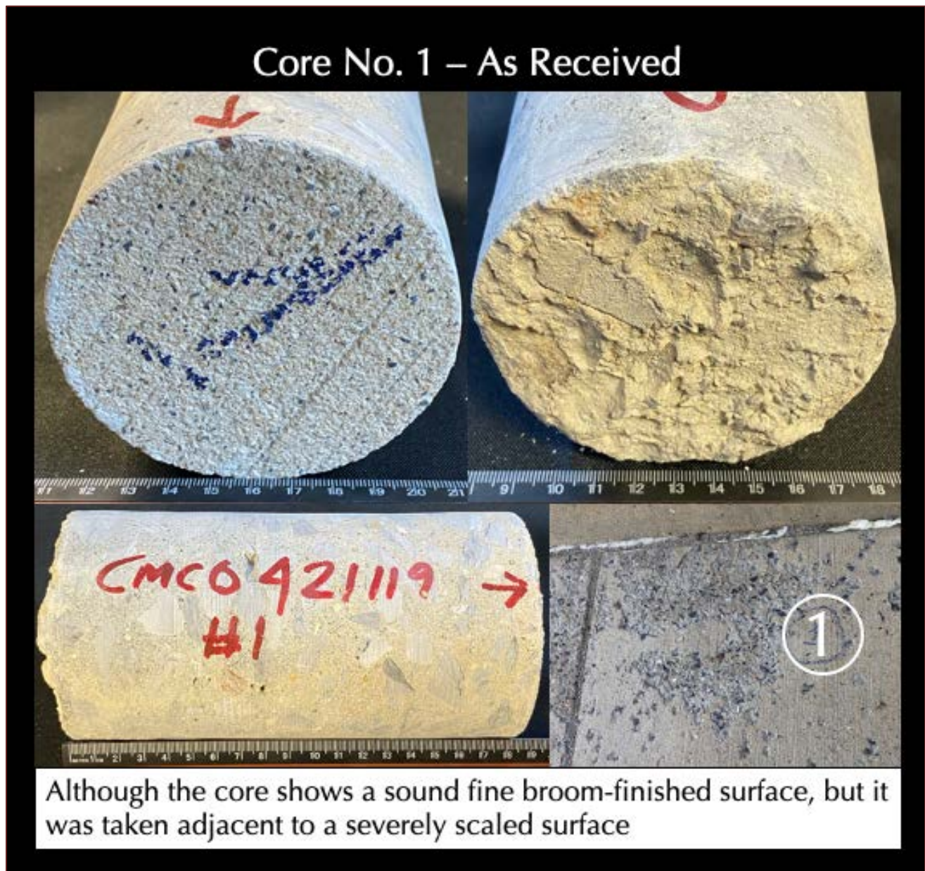
Figure 8: Core 1 as received showing fine broom-finished surface at the top left photo even though the core was taken from a scaled area (see Figures 1 and 3 and at the bottom right inset), bottom surface of core at the top right, and side cylindrical surface at the bottom left photo.
