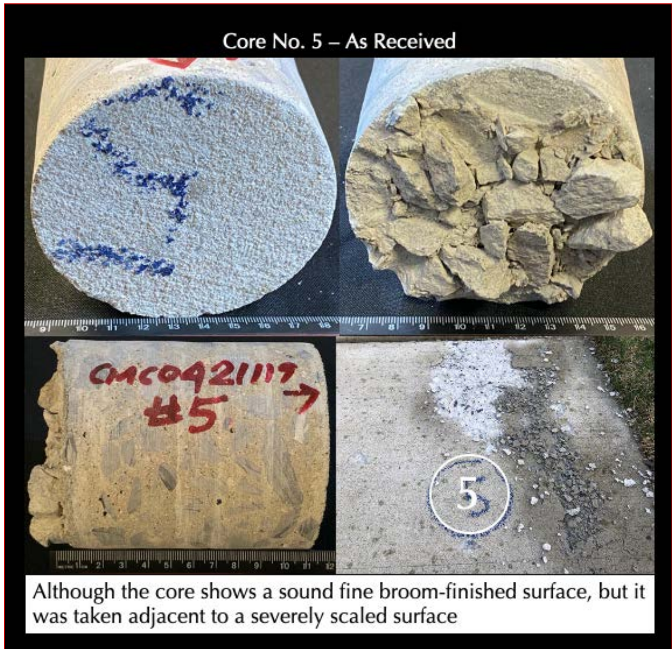
Figure 12: Core 5 as received showing sound fine broom-finished surface even though the core was taken from a scaled area as shown in the bottom right inset of field photo, bottom surface of core at the top right, and side cylindrical surface at the bottom left photo.
