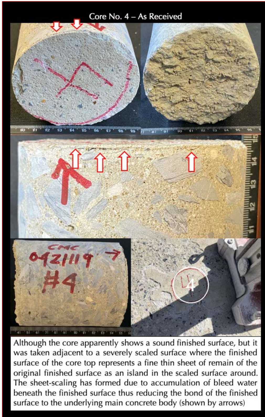
Figure 11: Core 4 as received showing thin sheet-style incipient scaling where the original finished surface is loosely adhered to the main body with a weak bond marked by arrows in the middle row, which is consistent with sheet-scaling at the core location at the bottom right inset due to accumulation of bleed water underneath the prematurely finished surface, bottom surface of core at the top right, and side cylindrical surface at the bottom left photo.
