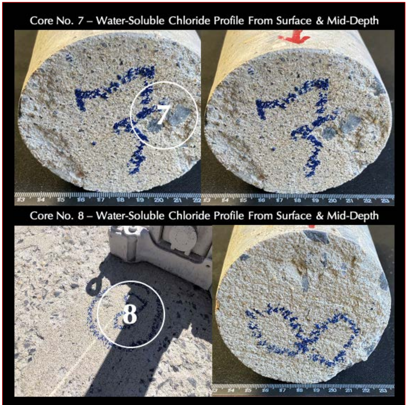
Figure 18: Water-soluble chloride contents of concrete were determined from the top distressed surface locations and at mid-depth locations of Cores 7 and 8.
