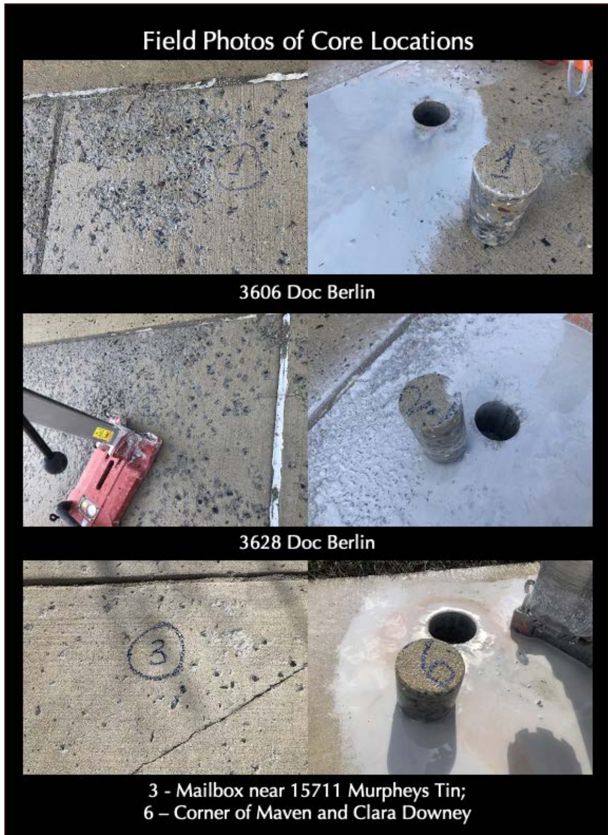
Figure 2: Field photographs showing surface scaling of concrete slab surface at the locations of Cores 1, 2, 3, and 6.
