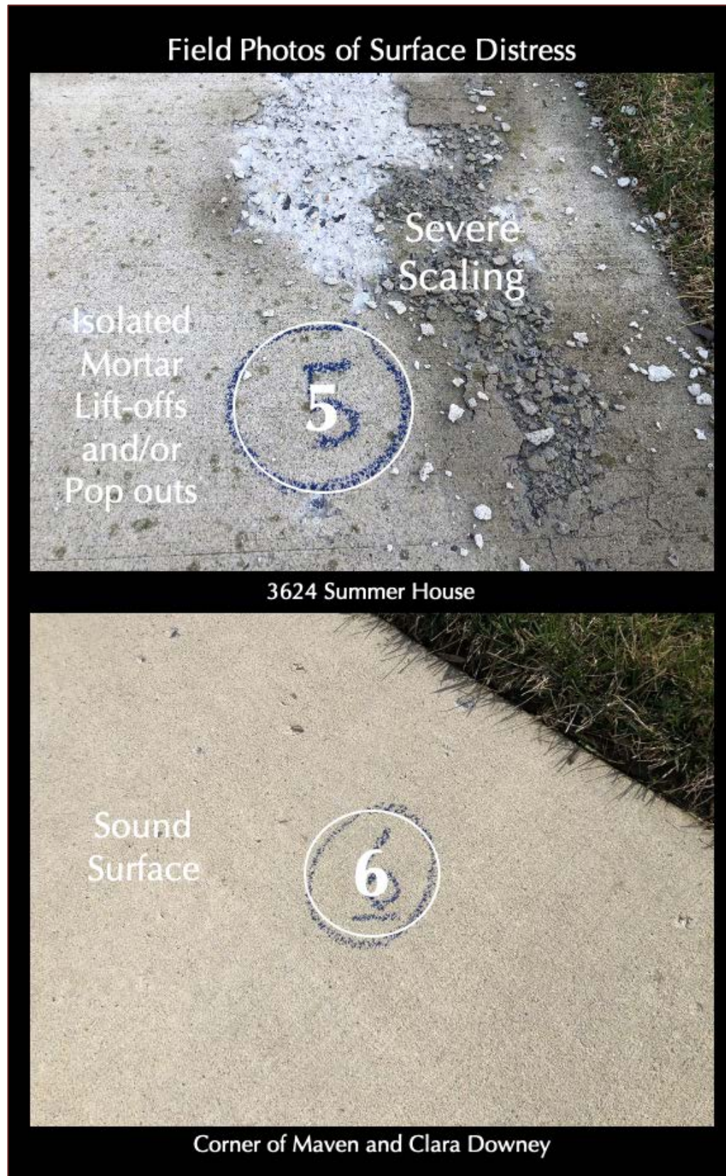
Figure 6: Severe scaling at the location of Core 5 whereas sound visually distress-free surface at the location of Core 6.
