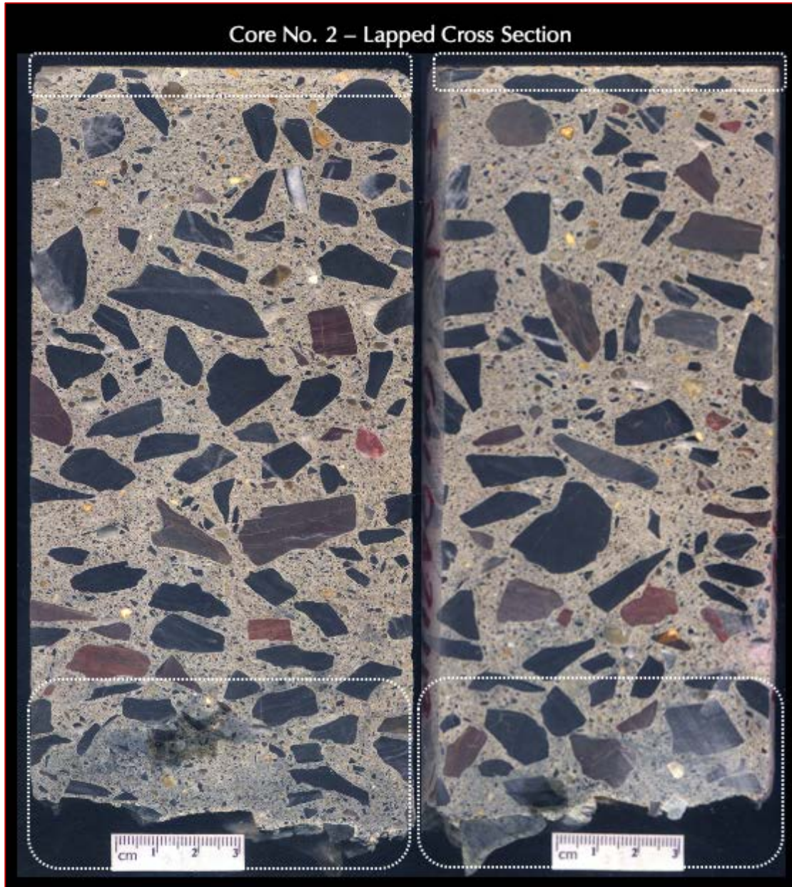
Figure 21: Two parallel lapped cross sections of Core 2 showing: (a) lightened gray toned paste at the top 5 to 6 mm of exposed surface (boxed) compared to relatively darker toned paste in the interior body, which occurs due to addition of water during finishing operations and/or finishing in the presence of bleed water at the surface, either practice would increase the porosity and water-cementitious materials ratio of paste and decrease the wear resistance and durability of exposed surface; (b) crushed limestone coarse aggregate particles, which are well-graded but show slight segregation at the top inch of the finished surface; (c) overall dense, and well-consolidated nature of concrete in the body; and greenish-gray discoloration of paste at the bottom 1 to 2 inches (boxed) due to the presence of ground granulated blast furnace slag as a cementitious component in the paste.
