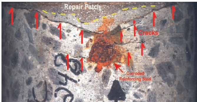
Fig. 2: Side view of a core showing ineffective repair patches and continued corrosion of the reinforcing steel in the concrete
