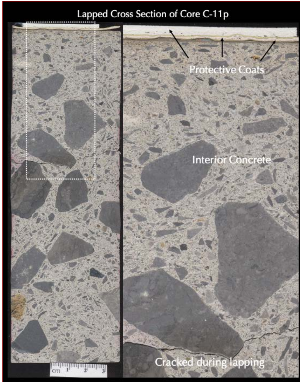
Figure 9: Lapped cross section at left and an enlarged view of the boxed area of lapped cross section at the right of Core C-11p. Notice the overall dense and well-consolidated nature of concrete in both sections containing dense, dark gray, crushed limestone coarse aggregate, where the coarse particles are poorly graded due to the deficiency of some intermediate and finer size fractions. The fine aggregate is a mixture of crushed limestone, marine shell fragments, and finer-size crushed siliceous fragments (quartz, feldspar, chert, quartzite, siltstone, etc.), which are well-graded and well-distributed throughout the depth of the core. Notice a series of protective coats applied on the exposed side of concrete to protect the concrete from penetration of potentially deleterious agents (chloride, carbon dioxide, moisture, etc.) from the marine environment.
