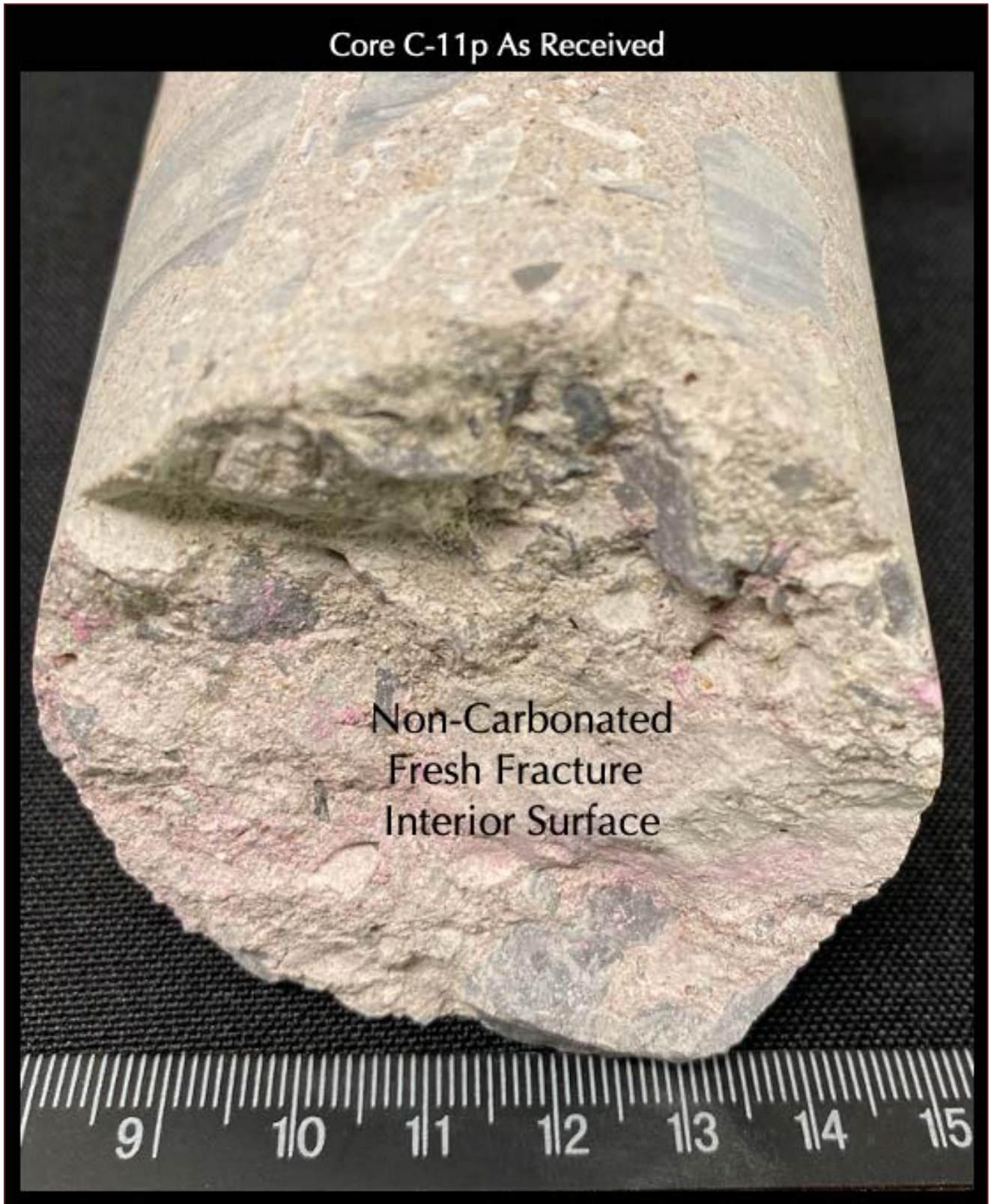
Figure 3: Fresh fractured interior opposite end of Core C-11p with a pinkish-discoloration due to field test of carbonation with phenolphthalein alcoholic solution.
