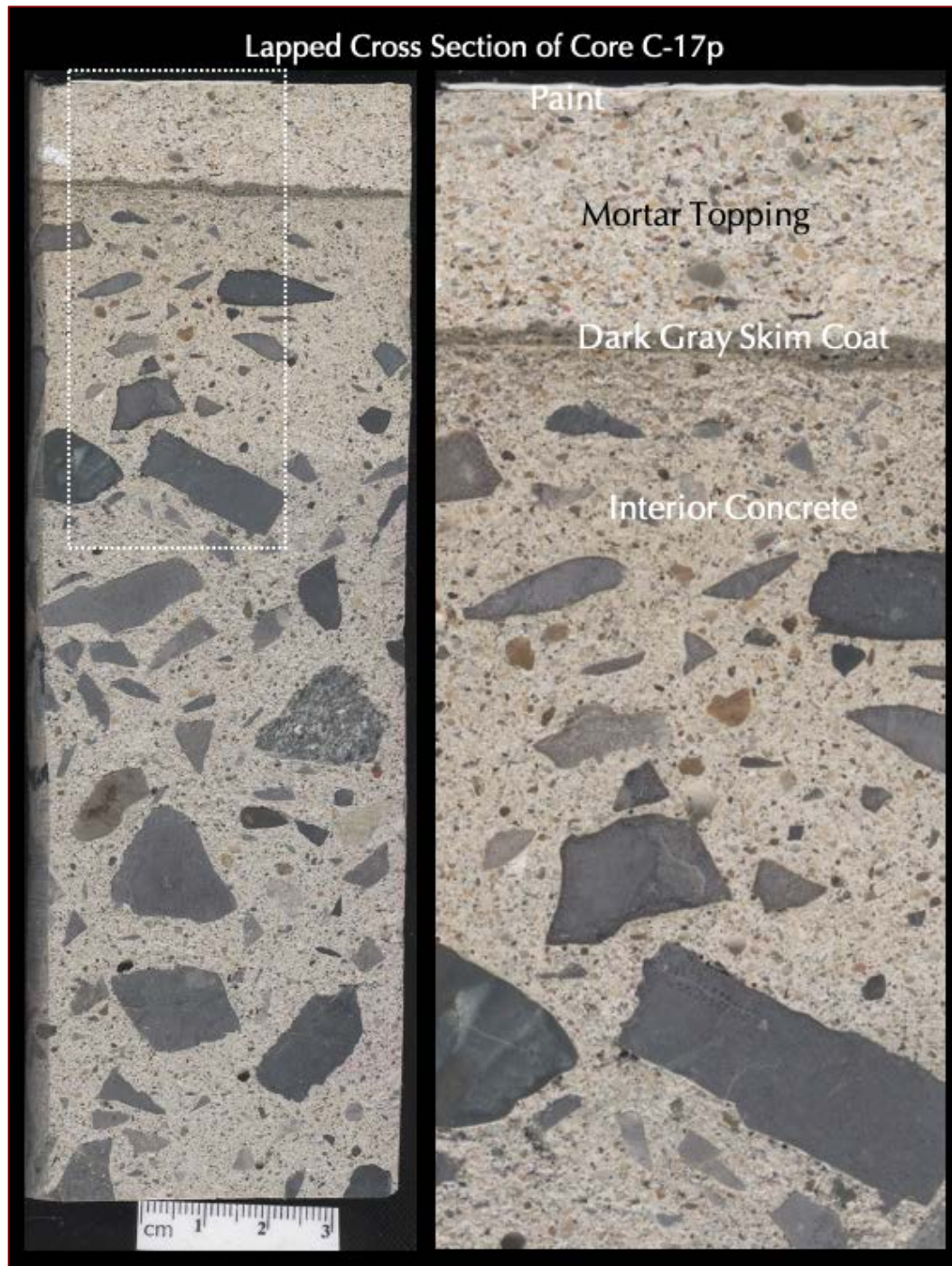
Figure 10: Lapped cross section at left and an enlarged view of the boxed area of lapped cross section at the right of Core C-17p. Notice the overall dense and well-consolidated nature of concrete in both sections containing dense, dark gray, crushed limestone coarse aggregate, where the coarse particles are poorly graded due to the deficiency of some intermediate and finer size fractions. The fine aggregate is a mixture of crushed limestone, marine shell fragments, and finer-size crushed siliceous fragments (quartz, feldspar, chert, quartzite, siltstone, etc.), which are well-graded and well-distributed throughout the depth of the core. Notice a series of protective coats sandwiched between a thick mortar coat, all applied on the exposed side of concrete to protect the concrete from penetration of potentially deleterious agents (chloride, carbon dioxide, moisture, etc.) from the marine environment.
