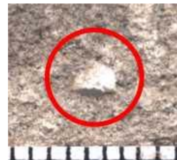
Shown is a white lump of hydrated lime in a portland cement-lime mortar. The bars are at \frac{1}{16} -in. intervals.
