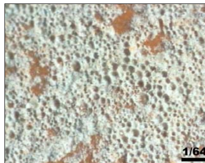
Too much air gives a frothy texture of paste and reduces the strength
