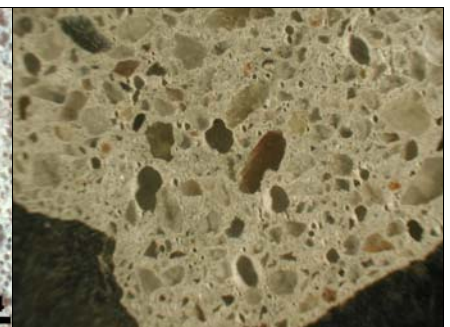
Too little air reduces the freeze-thaw resistance of concrete
