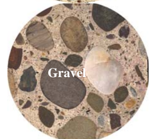
Commonly found aggregates in concrete
